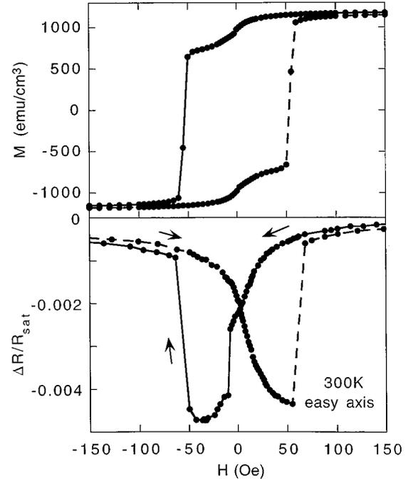
FIG. 3. Magnetoresistance effect  $\Delta R/R_{\text{sat}}$  with  $R_{\text{sat}} = R(H_{\text{max}} = 500 \text{ Oe})$  and magnetization measured at 300 K with a field applied along the easy axis for a  $\text{Co}_{65}\text{Fe}_{35}/\text{Ag}/(\text{Co}_{65}\text{Fe}_{35})_{50}\text{Gd}_{50}$  (100 Å/80 Å/100 Å) trilayer (glass substrate).
