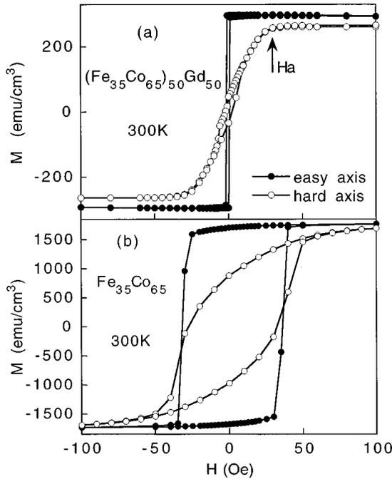
FIG. 1. Hysteresis cycles obtained at 300 K for 100 Å-thick amorphous  $(\text{Co}_{65}\text{Fe}_{35})_{50}\text{Gd}_{50}$  (a) and polycrystalline  $\text{Co}_{65}\text{Fe}_{35}$  (b) alloys deposited on amorphous Si (glass substrate).
