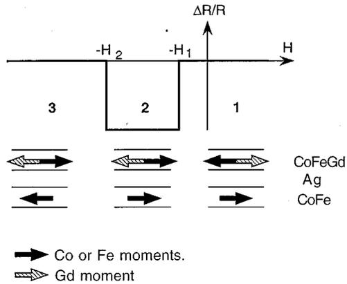
FIG. 4. Illustration of the negative spin-valve effect.
