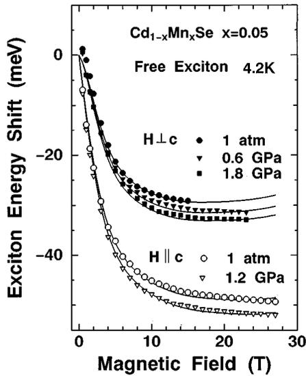
FIG. 3. Field-induced energy shift of the A exciton photoluminescence line in  $\text{Cd}_{0.95}\text{Mn}_{0.05}\text{Se}$  under several pressures. Experimental and theoretical values are shown by markers and solid lines, respectively.
