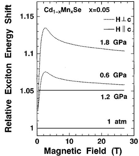
FIG. 9. Theoretical field-induced shift of the energy of the A exciton at several pressures relative to the shift at 1 atm in  $\text{Cd}_{0.95}\text{Mn}_{0.05}\text{Se}$  for  $H \parallel c$  (solid lines) and  $H \perp c$  (dashed lines).
