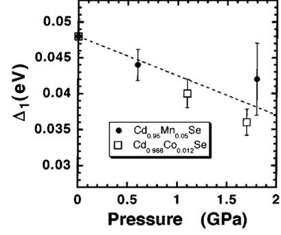
FIG. 6. Pressure dependence of the crystal field anisotropy energy  $\Delta_1$  in  $\bullet$   $\text{Cd}_{0.95}\text{Mn}_{0.05}\text{Se}$  and  $\square$   $\text{Cd}_{0.988}\text{Co}_{0.012}\text{Se}$ . The dotted line shows the linear least-squares fit to the experimental data.
