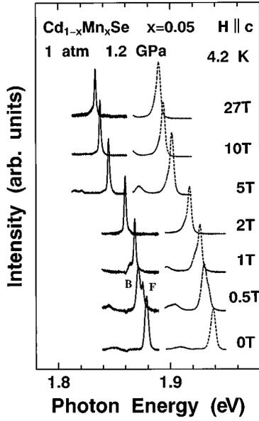
FIG. 2. Photoluminescence spectra due to the A exciton in  $\text{Cd}_{0.95}\text{Mn}_{0.05}\text{Se}$  under various magnetic fields at 1 atm and 1.2 GPa. The features due to free and bound excitons are denoted as  $F$  and  $B$ , respectively.
