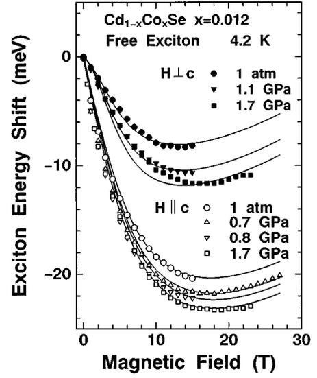
FIG. 4. Field-induced energy shift of the A exciton photoluminescence line in  $\text{Cd}_{0.988}\text{Co}_{0.012}\text{Se}$  under several pressures. Experimental and theoretical values are shown by markers and solid lines, respectively.
