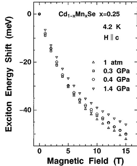
FIG. 5. Field-induced energy shift of the A exciton photoluminescence line in  $\text{Cd}_{0.75}\text{Mn}_{0.25}\text{Se}$  under several pressures.
