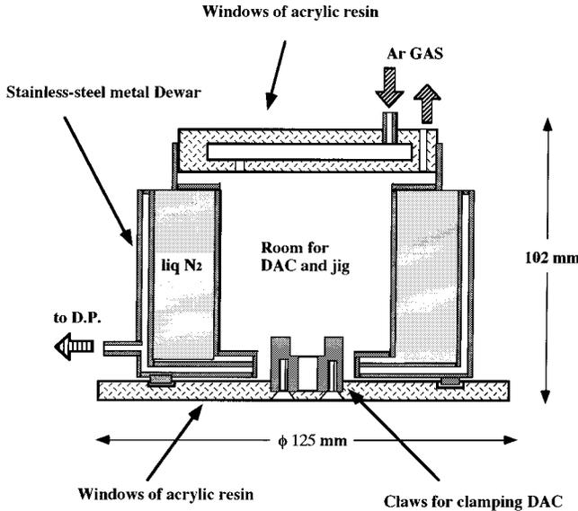
FIG. 1. Schematic diagram of an apparatus to liquefy argon in a clamp-type diamond anvil cell.
