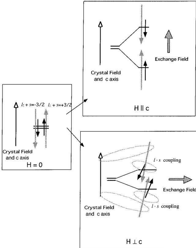
FIG. 8. A schematic representation of the orientation of spin (solid arrows) and angular (shaded arrows) momentum of the A valence band under magnetic field relative to the rotation axis (open arrows) of the trigonal crystal field.
