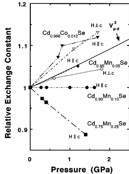
FIG. 7. Pressure-induced change of the exchange constant  $|N_0\beta_{\text{hyb}}|$  in  $\text{Cd}_{0.95}\text{Mn}_{0.05}\text{Se}$ ,  $\text{Cd}_{0.75}\text{Mn}_{0.25}\text{Se}$ , and  $\text{Cd}_{0.988}\text{Co}_{0.012}\text{Se}$ . Previous experimental results for  $\text{Cd}_{0.90}\text{Mn}_{0.10}\text{Se}$  (Ref. 6) are also shown for comparison. The continuous line shows the pressure dependence of the squared  $p$ - $d$  transfer integral  $V_{pd}^2$ .
