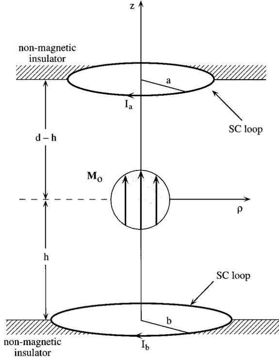
FIG. 1. The magnetic sphere of radius  $a$  is trapped between two superconducting rings of radii  $a$  and  $b$  and fixed separation  $d$ , carrying induced currents  $I_a$  and  $I_b$ . The levitation height  $h$  is measured from ring  $b$ .
