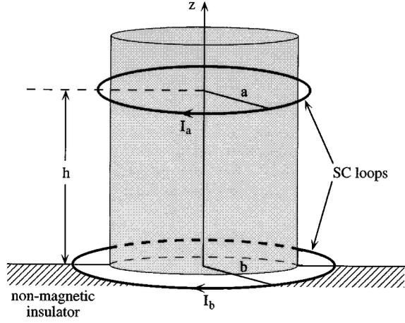
FIG. 11. Superconducting ring current  $I_a$  levitated by a fixed SC ring with current  $I_b$ .
