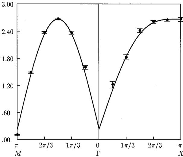
FIG. 3. The spin-flip excitation spectrum in  $\bullet$  and in units of  $J$ , calculated on a  $12 \times 12$  lattice, along the (1,0) (right-hand side) and the (1,1) axes. The curve corresponds to the renormalized spin-wave result with  $Z_r = 1.22$  and an up-shift  $\cong 0.22$  (presumably due to the finite lattice size).
