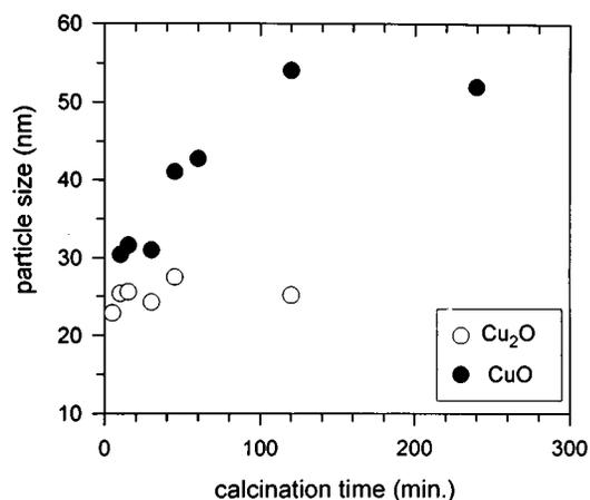
FIG. 1. Dependence of the particle size (coherently diffracting XRD domain size) of CuO and Cu<sub>2</sub>O phases on the calcination time of the copper citrate precursor produced by rapid dehydration. All the samples were calcined at 400 °C.
