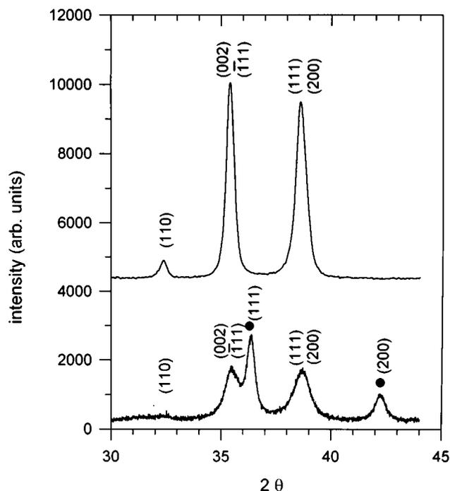
FIG. 3. X-ray diffractograms from samples prepared by the calcination of copper citrate precursors at 250 °C for 15 min (lower curve) and 350 °C for 15 min (upper curve). The upper spectrum shows the characteristic diffraction maxima for CuO only, while the lower one shows lines from CuO as well as Cu<sub>2</sub>O (marked with ●).
