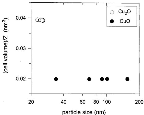
FIG. 4. Variation of the normalized unit-cell volume (per formula unit) with the XRD domain size in the CuO-Cu<sub>2</sub>O system.
