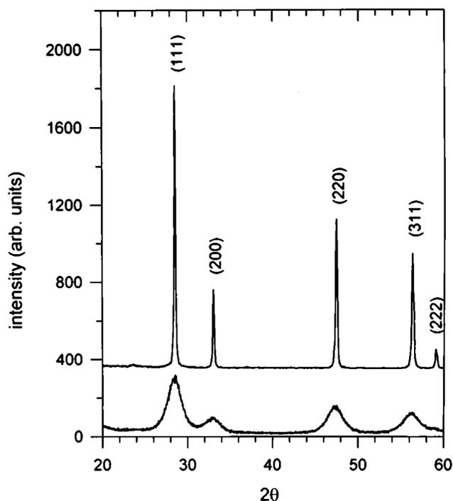
FIG. 5. X-ray diffractograms for CeO<sub>2</sub> samples produced by calcining the precursor at 100 °C for 15 min (lower curve) and 1000 °C for 10 h (upper curve). The upper spectrum represents single phase, bulk CeO<sub>2</sub> ( $d_{\text{BET}}=684$  nm), and there is no observable phase change down to 4.8 nm ( $d_{\text{BET}}$ ) as can be seen from the lower spectrum.
