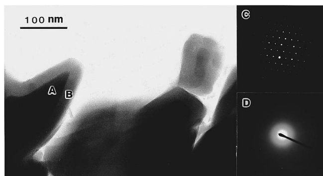
FIG. 1. TEM bright-field image and electron-diffraction patterns from crushed coesite grains after annealing at 1200 K for 1.5 h showing amorphous layer formation at the surface. Diffraction patterns C and D were taken from the areas marked A and B in the bright-field image, respectively.
