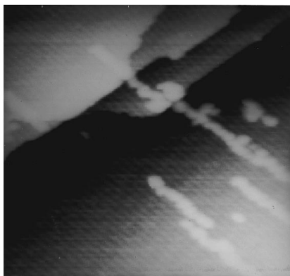
FIG. 8. Image of 600 \text{ \AA} \times 600 \text{ \AA} of the Pt(100) surface showing several steps perpendicular to the reconstruction rows. Sm has been evaporated for 1 min at an estimated rate of 0.15 \text{ \AA}/\text{min} . The step edges do not seem to act as nucleation centers for the Sm-Pt islands, as the islands are seen to have nucleated on both the lower terrace (lower right half of the figure) as well as at the steps (upper left corner).
