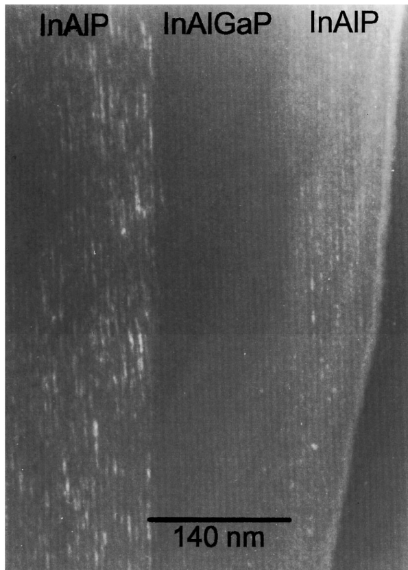
FIG. 3. Transmission electron microscopy dark-field image of InAlP/InAlGaP/InAlP heterostructure. Ordered domains (white linear features) are clearly seen in the lower barrier InAlP layer, and end abruptly at the InAlGaP active layer.
