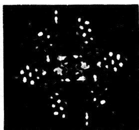
FIG. 2. (a), (b) STM images ( 136 \text{ \AA} \times 136 \text{ \AA} ) of the (4\sqrt{3} \times 4\sqrt{3}) R30^\circ structure [hexagonal structure (Ref. 37)]; (a) empty-state (2500 mV, 20 nA) image with a (4\sqrt{3} \times 4\sqrt{3}) unit cell superimposed on; (b) filled state (-2500 mV, 20 nA). (c) LEED pattern (51 V) of the structure. (d) FFT of (a).
