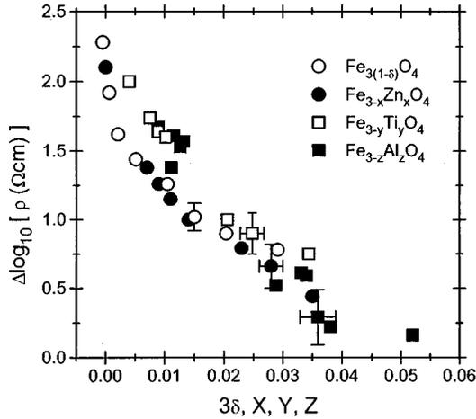
FIG. 6. Resistivity drop near the Verwey transition,  $\Delta \log_{10} \rho$  vs dopant concentration and nonstoichiometry.
