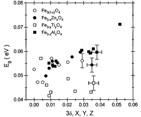
FIG. 7. Plot of activation energy as a function of concentration (or nonstoichiometry) for some weakly doped magnetite-based compounds.
