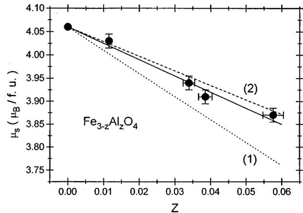
FIG. 5. Variation of saturation moment at 4.2 K with composition parameter  $z$  for various models of cationic distribution cited in the literature (line 1, Refs. 14 and 15, line 2, Ref. 16); solid circles represent measured data points, while solid line is the best fit to these data.
