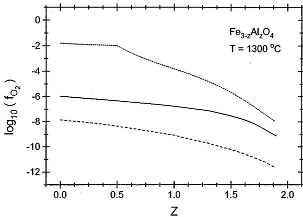
FIG. 2. Experimentally determined (Ref. 25) stability field at 1300 °C for  $\text{Fe}_{3-z}\text{Al}_z\text{O}_4$  (dashed lines) and intrinsic oxygen fugacity of stoichiometric aluminum ferrites calculated after Eq. (3) (solid line).
