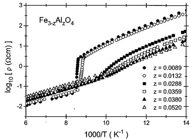
FIG. 3. Variation of resistivity  $\rho$  with temperature for selected samples in the vicinity of the Verwey transition.
