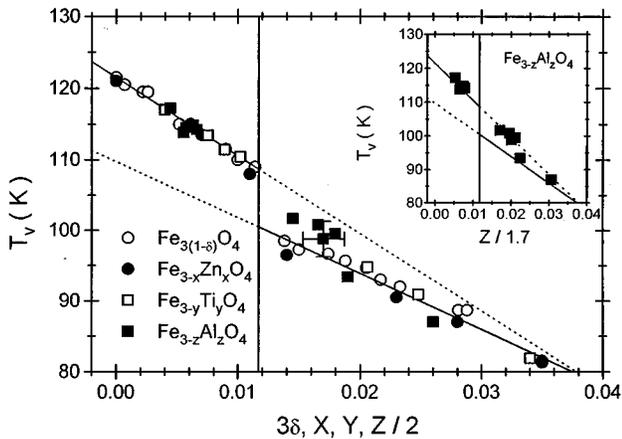
FIG. 4. Dependence of the Verwey transition temperature with composition, with  $z/2$  scaling for aluminum ferrites. The inset shows yet another scaling for  $\text{Fe}_{3-z}\text{Al}_z\text{O}_4$  with the results for other ferrites marked as a solid line.
