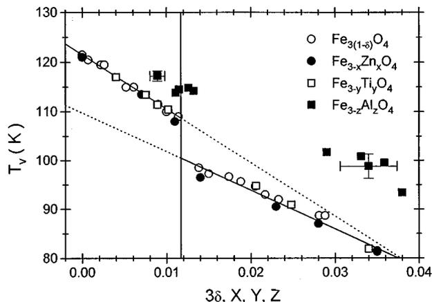
FIG. 1. Dependence of the Verwey transition temperature  $T_v$  on composition and on oxygen stoichiometry. The regions of first- and higher order are clearly delineated (data for nonstoichiometric or Zn- and Ti-doped magnetite cited after Ref. 5).
