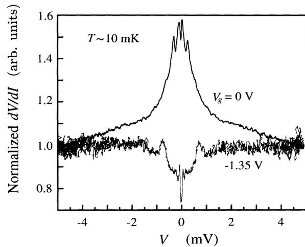
FIG. 3. Measured  $dV/dI$ - $V$  characteristics for another junction with  $L=0.3 \mu\text{m}$ . The resistance of the constriction  $R_C$  obtained from the measured  $R_N$  for  $V_g=-1.35$  V corresponds to the seventh quantized conductance step in a quantum point contact.
