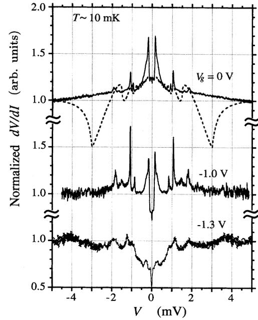
FIG. 2. Measured differential resistance-voltage ( $dV/dI-V$ ) characteristics as a function of gate voltage  $V_g$ . The  $dV/dI$  is normalized by the junction normal resistance  $R_N$  and is unity at  $V = \pm 5$  mV. The dotted curve represents the calculated one based on the OTBK theory.
