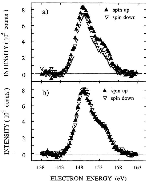
FIG. 1. Spin-resolved sulfur  $L_{2,3}VV$  Auger-electron spectra from the  $c(2 \times 2)$ S/Fe(001) system [majority spin ( $\blacktriangle$ ) and minority spin ( $\nabla$ )]. Electron emission angles are (a)  $\theta = +10^\circ$ , and (b)  $\theta = +2.5^\circ$ .
