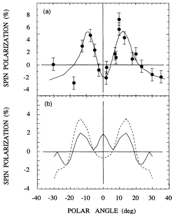
FIG. 2. (a) Measured spin polarization of the  $L_{2,3}VV$  Auger-electron diffraction pattern (SPAED) for the main peak (the line is a guide to the eye). The polar angle scan is measured in the (100) plane. (b) Calculated sulfur  $L_{2,3}VV$  SPAED pattern for two different surface Fe layer magnetizations: equal to the Fe bulk magnetization (full line) and magnetically dead (dashed line).
