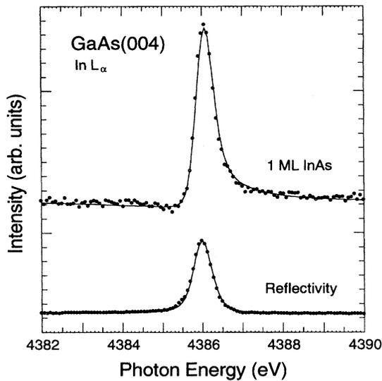
FIG. 1. Photon-energy dependence of the reflectivity (lower) and the In- $L_{\alpha}$  fluorescence yield (upper) near the GaAs(004) Bragg backreflection condition. The solid lines are the best fits to the data points (see text).
