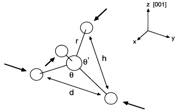
FIG. 3. An InAs tetrahedron under compressive strain in the  $x$ - $y$  plane with equivalent near-neighbor bond lengths  $r$ . Here  $z$  is the  $[001]$  direction. The in-plane and out-of-plane second-neighbor distances are  $d = 2r \sin(\theta/2)$  and  $h = 2r \sin(\theta'/2)$ .
