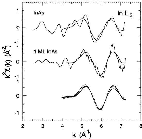
FIG. 2.  $k^2$ -weighted  $\text{In-}L_3$  EXAFS,  $k^2\chi(k)$ , from the InAs monolayer (middle) and the bulk InAs standard (upper). Superimposed on the data are the Fourier-filtered first-shell contributions, which correspond to the In-As near-neighbor bond. The lower portion of the figure shows the fit (solid line) to the filtered data from the InAs monolayer (see text).
