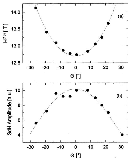
FIG. 4. (a) Angular dependence of the magnetic field giving the 13th peak in the MR oscillations. (b) Angular dependence of the oscillation amplitude for the 13th peak fitted by the LK formula for a cylindrical FS (dashed curve).
