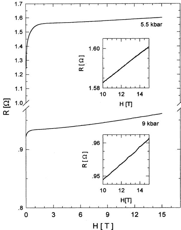
FIG. 1. Interlayer resistance of  $\kappa$ -(BEDT-TTF)<sub>2</sub>Cu[N(CN)<sub>2</sub>]Br vs magnetic field at various pressures at 1.45 K. The magnetic field is applied normal to the *ac* plane.
