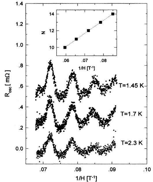
FIG. 2. Oscillatory component  $R_{\text{osc}}$  of MR vs inverse magnetic field  $1/H$  at different temperatures. Inset shows the resistance peak periodicity vs inverse magnetic field, where  $N$  is the number of the peak.
