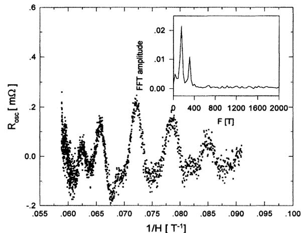
FIG. 3. Oscillatory component  $R_{\text{osc}}$  of MR vs  $1/H$  up to 17 T at 1.45 K. Inset shows the fast Fourier transformation.
