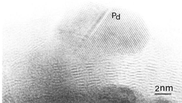
FIG. 2. High-resolution transmission electron microscopy picture showing a Pd nanocrystal in the upper right corner. An internal twin boundary is visible in the nanocrystal.
