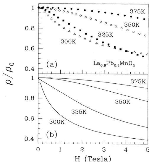
FIG. 4. (a) Magnetic field dependence of the resistivity for the same  $\text{La}_{0.6}\text{Pb}_{0.4}\text{MnO}_{3-\delta}$  crystal as in Fig. 3. The resistivities are normalized by the respective zero-field values. (b) Theoretical fit for the two-component lattice polaron model discussed in the text.
