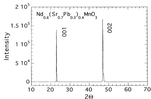
FIG. 1. X-ray diffraction pattern of a  $\text{Nd}_{0.6}(\text{Sr}_{0.7}\text{Pb}_{0.3})_{0.4}\text{MnO}_{3-\delta}$  single crystal. The reflections ( $hkl$ ) are indexed as shown.
