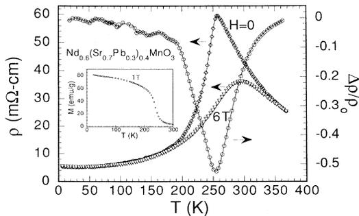
FIG. 2. Temperature dependence of the electrical resistivity and magnetoresistance  $\frac{R(6\text{ T})-R(0\text{ T})}{R(0\text{ T})}$  for a single crystal of  $\text{Nd}_{0.6}(\text{Sr}_{0.7}\text{Pb}_{0.3})_{0.4}\text{MnO}_{3-\delta}$ . The inset shows the magnetization  $M$  versus temperature at  $H = 1\text{ T}$  for the same crystal.
