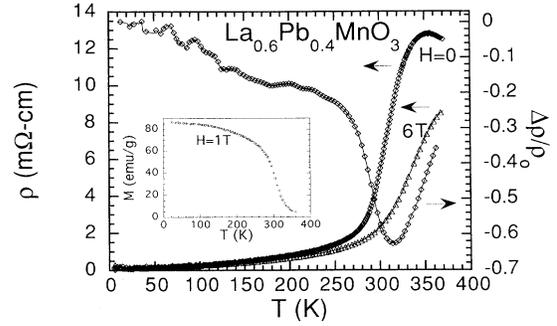
FIG. 3. Temperature dependence of the electrical resistivity and magnetoresistance  $\frac{R(6\text{ T})-R(0\text{ T})}{R(0\text{ T})}$  for a single crystal of  $\text{La}_{0.6}\text{Pb}_{0.4}\text{MnO}_{3-\delta}$ . The inset shows the magnetization  $M$  versus temperature for an applied field of 1 T for the same crystal.
