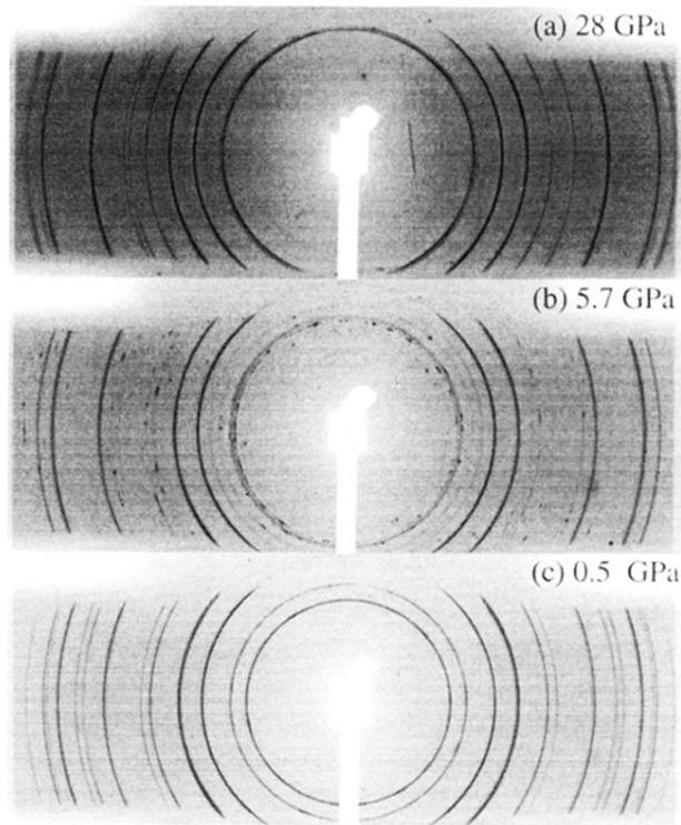
FIG. 3. X-ray-diffraction images of Ce metal mixed with the Cu pressure standard during decompression. (a) The diffraction rings are continuous and uniform in intensity for the bct phase at 28 GPa. (b) The spotty rings show the orientation effects in the  $\alpha$ -U phase. (c) The rings become continuous and uniform again during back transformation to the fcc phase. Note that the Cu diffraction rings are always continuous through the decompression cycle.
