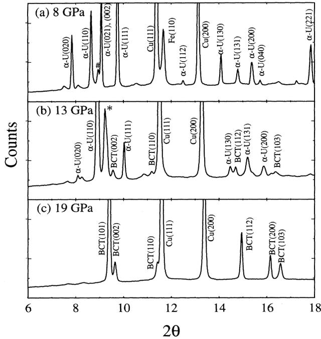
FIG. 2. The radially integrated diffraction patterns of the Ce with  $\lambda=0.4066 \text{ \AA}$ . (a) At 8 GPa the pattern is fitted to the  $\alpha$ -U structure [the peak with the # label is from residual fcc(111)]. (b) At 13 GPa the bct phase emerges and coexists with the  $\alpha$ -U phase [the peak with the \* label is the mixture of  $\alpha$ -U(021), (002), and bct(101)]. (c) The single phase bct diffraction pattern is shown at 19 GPa.
