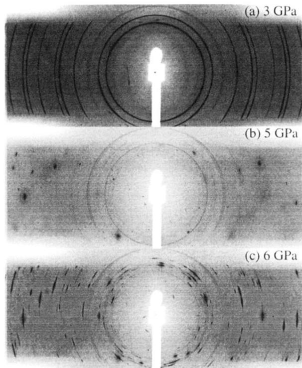
FIG. 1. X-ray-diffraction images of pure Ce metal at 3 GPa, 5 GPa, and 6 GPa, respectively. (a) At 3 GPa, the sample is in the fcc phase. (b) At 5 GPa, the large grain size of the  $\alpha$ -U phase is indicated by only a few diffraction spots. The weak ring patterns are from the residual fcc phase. (c) The orientation effects decrease gradually at higher pressure, and rings tend to become continuous.
