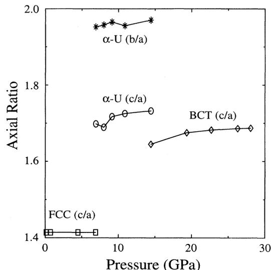
FIG. 4. The axial ratio of the various phases as a function of pressure in Ce. The fcc phase data are shown with a constant value of  $c/a = 1.414$ . The axial ratios for the  $\alpha$ -U phase are relatively insensitive to pressure. The  $c/a$  ratio for the bct phase increases with pressure and tends to saturate at high pressure.
