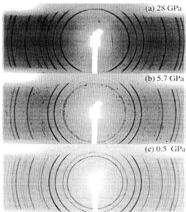
FIG. 3. X-ray-diffraction images of Ce metal mixed with the Cu pressure standard during decompression. (a) The diffraction rings are continuous and uniform in intensity for the bct phase at 28 GPa. (b) The spotty rings show the orientation effects in the  $\alpha$ -U phase. (c) The rings become continuous and uniform again during back transformation to the fcc phase. Note that the Cu diffraction rings are always continuous through the decompression cycle.
