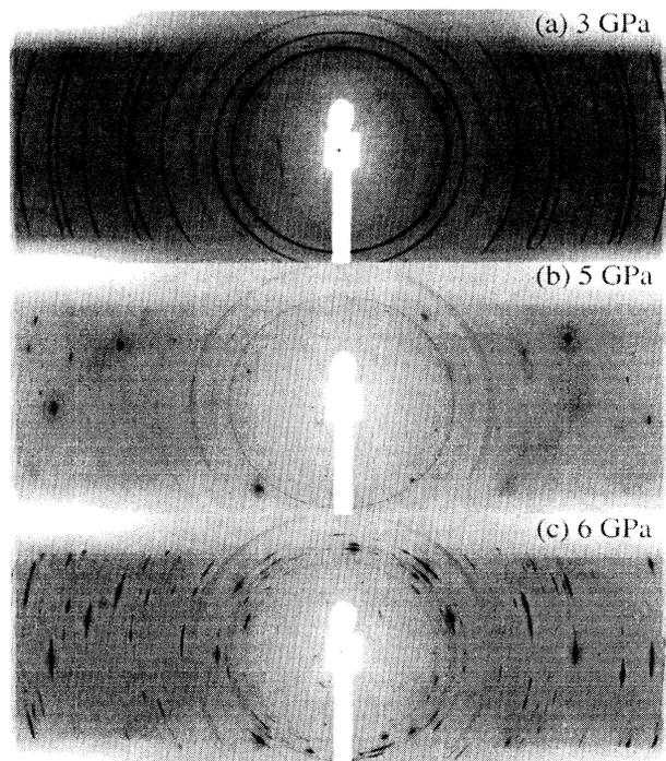
FIG. 1. X-ray-diffraction images of pure Ce metal at 3 GPa, 5 GPa, and 6 GPa, respectively. (a) At 3 GPa, the sample is in the fcc phase. (b) At 5 GPa, the large grain size of the  $\alpha$ -U phase is indicated by only a few diffraction spots. The weak ring patterns are from the residual fcc phase. (c) The orientation effects decrease gradually at higher pressure, and rings tend to become continuous.
