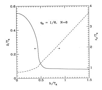
FIG. 1. The solution of the saddle-point equations in the magnetic field for  $q_0 = 1/6$  and N = 6.  $T_K$  is defined by (38).  $\epsilon_f$  is the position of the resonant level and  $\Delta$  is the width.
