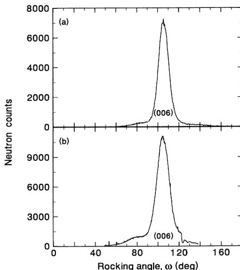
FIG. 2. Rocking curves of the (006) reflections of (a) the C<sub>24</sub>Rb sample at room temperature using  $\lambda = 0.245$  nm and  $2\theta = 31.7^\circ$ . (b) Same sample at 120 K (using  $\lambda = 0.240$  nm and  $2\theta = 31.0^\circ$ ) after “inserting” N<sub>2</sub>. The deduced mosaic spreads are  $\Delta\phi = 11.0^\circ$  and  $14.0^\circ$ , respectively.
