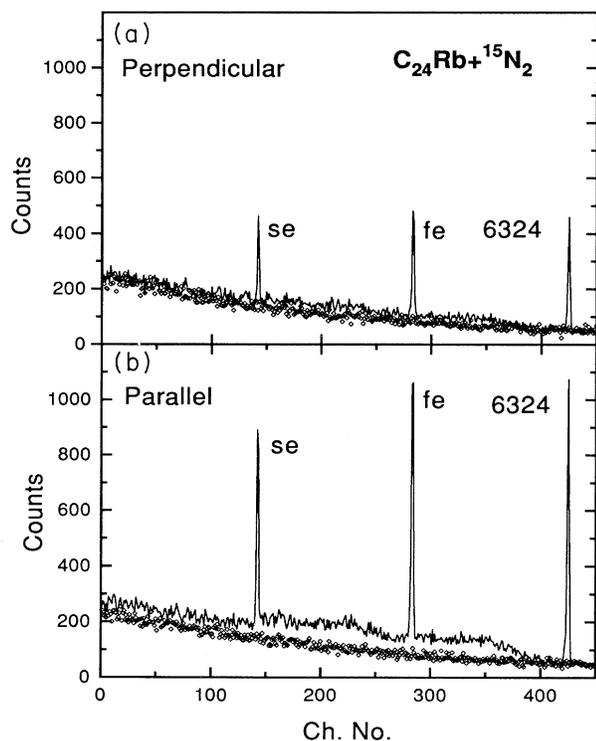
FIG. 3. Sum of scattered radiation spectra obtained at  $T=12-70$  K, from  $^{15}N_2$  physintercalated in a  $C_{24}Rb$  sample and using a  $150\text{-cm}^3$  HPGe detector with the beam parallel and perpendicular to the graphite planes. The “background” scattered spectra were obtained by evacuating the  $^{15}N_2$  gas from the container. The three peaks correspond to the photopeak, first escape (fe), and second escape (se) peaks of the resonantly scattered 6324-keV  $\gamma$  line.
