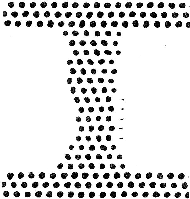
FIG. 9. The contact at N = 220 in the 250 K simulation. Layers 4 to 8 (indicated by the arrows) from the bottom of the contact have nearly identical atomic geometries.
