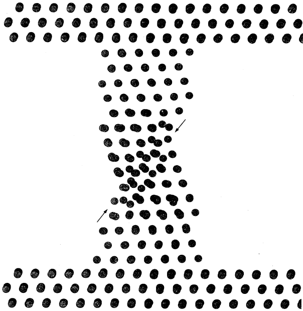
FIG. 5. The contact at N = 193 in the 10 K simulation. Observe the stacking fault (indicated by the arrows) running across the contact. This stacking fault gives rise to the scattering responsible for the trough in the tight-binding conductance.
