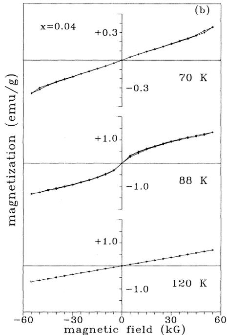
FIG. 8. The magnetization curves of  $U(Pd_{0.96}Fe_{0.04})_2Ge_2$  temperatures (a) 5, 20, and 50 K and (b) 70, 88, and 120 K.
