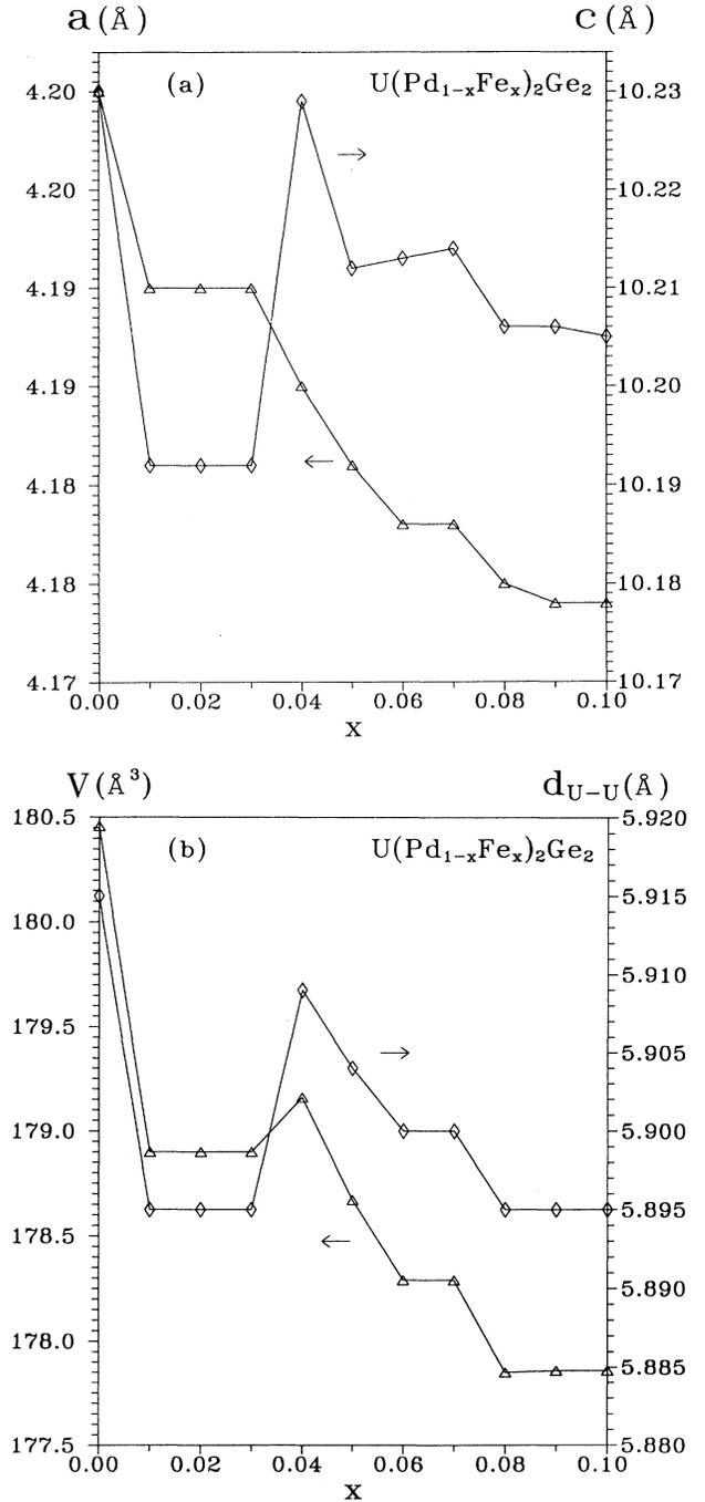
FIG. 1. The  $x$  dependence (a) of the crystal lattice parameters  $a$  and  $c$ , and (b) of the unit cell volume  $V$  and the calculated interatomic distance  $d_{\text{U-U}}$  between the nearest U atoms.
