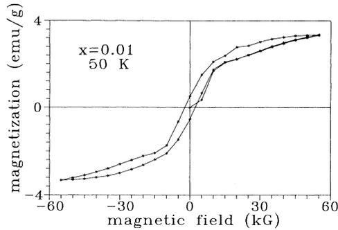
FIG. 6. The field dependence of the magnetization in  $U(Pd_{0.99}Fe_{0.01})_2Ge_2$  at 50 K.
