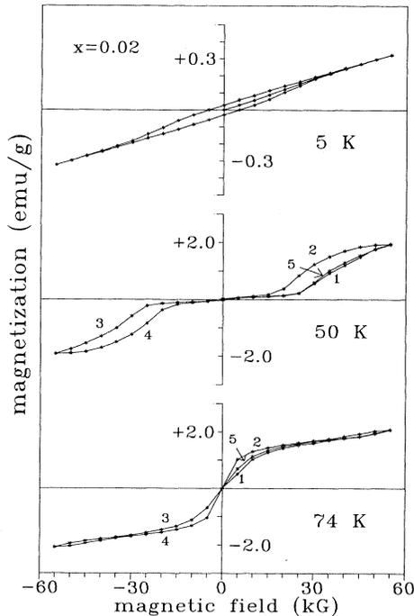
FIG. 7. The magnetization curves of  $U(Pd_{0.98}Fe_{0.02})_2Ge_2$  at different temperatures.
