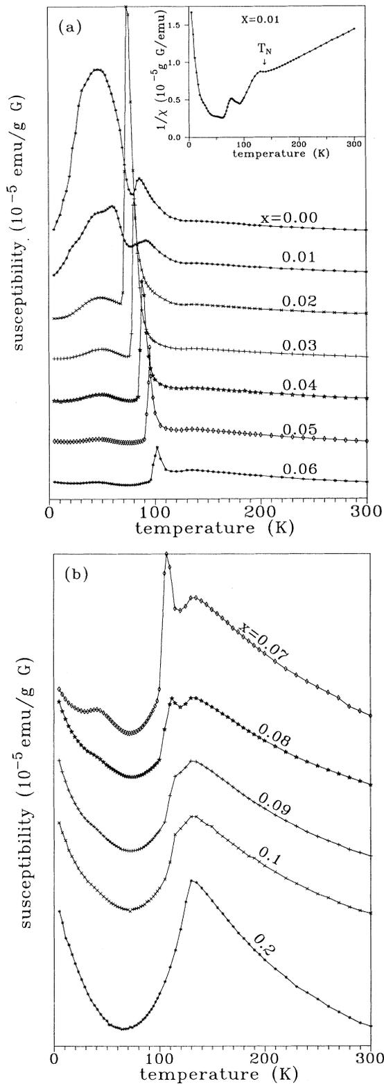
FIG. 2. The temperature dependence of the magnetic susceptibility in  $U(Pd_{1-x}Fe_x)_2Ge_2$  measured in an applied field of 2 kG: (a) for  $x=0.0-0.06$  and (b) for  $x=0.07-0.2$ . The inset in (a) shows the temperature dependence of the inverse magnetic susceptibility for  $x=0.01$ .
