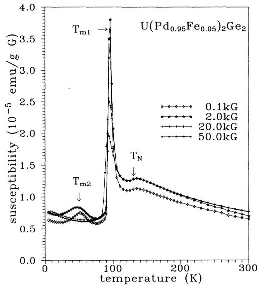
FIG. 4. The temperature dependence of the magnetic susceptibility of  $\text{U(Pd}_{0.95}\text{Fe}_{0.05})_2\text{Ge}_2$  in different applied fields  $H=0.1, 2, 20,$  and  $50$  kG.
