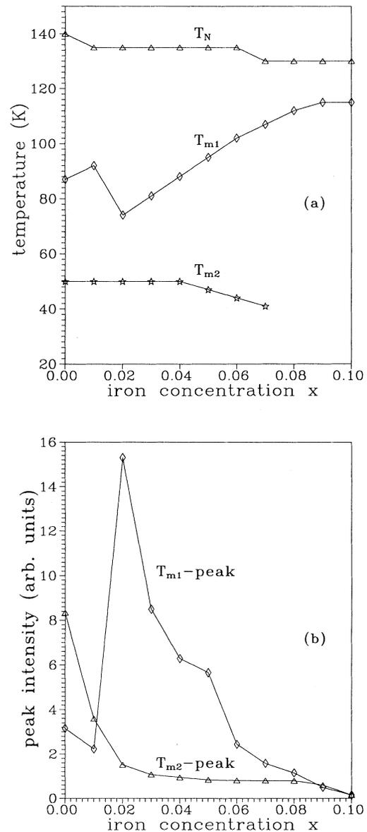
FIG. 3. The  $x$  dependence (a) of the magnetic transition temperatures  $T_N$ ,  $T_{m1}$ , and  $T_{m2}$  and (b) of the susceptibility peak intensities at the  $T_{m1}$  and  $T_{m2}$  points in  $U(Pd_{1-x}Fe_x)_2Ge_2$ .
