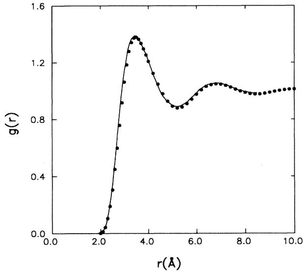
FIG. 6. Pure expectation result of the two-body radial distribution function (solid line) for liquid  ${}^4\text{He}$  at  $\rho_0^{\text{expt}}$  in comparison with the experimental data (points) of Ref. 25.
