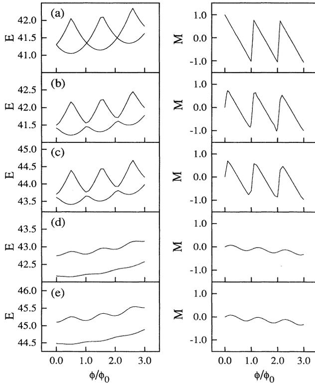
FIG. 2. The lowest two energy values and magnetization vs  $\Phi/\Phi_0$  for a four-electron system at  $\alpha = 20$ . (a) Noninteracting and impurity-free, (b) noninteracting, but with impurity potential ( $V_0 = 1.0, d = 0.2$ ), (c) interaction and impurity included ( $V_0 = 1.0, d = 0.2$ ), (d) noninteracting, but with impurity included ( $V_0 = 4.0, d = 0.5$ ), and (e) interaction and impurity included ( $V_0 = 4.0, d = 0.5$ ).
