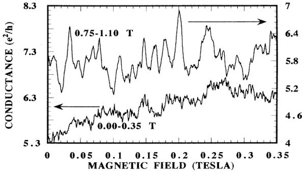
FIG. 2. Expanding the magnetic-field scale of Fig. 1(b) ( $W_e = 1.8 \mu\text{m}$ ,  $W = 0.74 \mu\text{m}$ ) to achieve greater sensitivity, a significant increase in both the average amplitude and period of the UCF is observed, as the magnetic field is increased.
