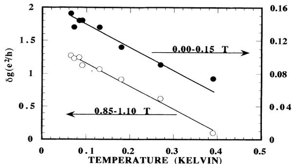
FIG. 8. Temperature dependence of the conduction fluctuations in a quantum wire, measured over two distinct magnetic-field ranges ( $W_e = 1.8 \mu\text{m}$ , and  $W = 1.22 \mu\text{m}$ ). For magnetic fields less than roughly 0.2 T the Landau levels are unresolved, while in the vicinity of 1 T distinct ScH oscillations are observed. The solid lines are straight-line fits to the data.
