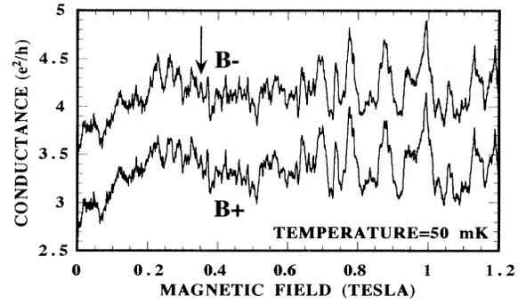
FIG. 3. Symmetry of the magnetoconductance of a quantum wire ( $W_e = 1.8 \mu\text{m}$ ,  $W = 0.55 \mu\text{m}$ ) with respect to field reversal. For the sake of clarity, the  $B$  trace has been shifted upwards by  $0.75e^2/h$ . The arrow marks the magnetic field at which the cyclotron orbit is calculated to be comparable to  $W$ .
