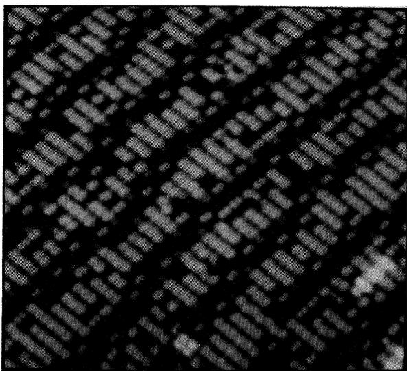
FIG. 4. Enlarged STM image of the Ni-contaminated Si(001)- $2 \times 1$  structure showing the details of line defects composed of dimer-vacancy defects. One of the two dimers adjacent to 2-DV is depressed and looks gray. The split-off dimer in (1+2)-DV is split into two regions forming a local  $1 \times 1$ -like structure. Sample bias voltage and tunnel current are  $-2.3$  V and  $0.5$  nA, respectively.
