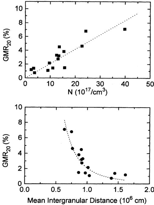
FIG. 12. Dependence of  $GMR_{20}$  on the total density of magnetic particles (above) and on the mean intergranular distance (below) for the  $Cu_{100-x}Co_x$  family. The dotted lines are guides for the eye.
