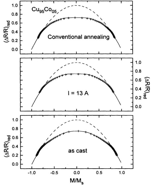
FIG. 13. Reduced GMR curves as functions of reduced magnetization for three selected samples of  $\text{Cu}_{95}\text{Co}_5$ . Crosses: experimental data; dashed lines: parabolic behavior predicted by the independent-moment model; full lines: present model [Eq. (28)]. A reduced number of experimental data is displayed. The fits were performed on the whole set of data.
