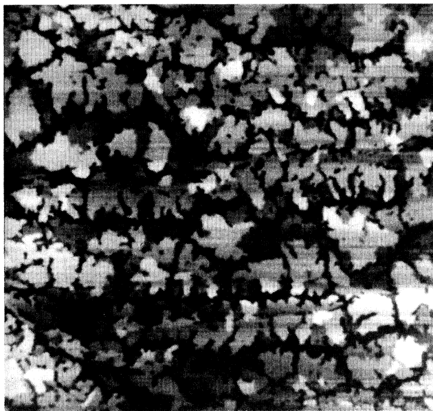
FIG. 2. Topographical force micrograph of a sample with a nominal coverage of 1.2 ML of C_{60} molecules, exhibiting dendritically shaped islands of up to 3 ML height. Scan size was 6.2 \times 6.2 \mu\text{m}^2 .
