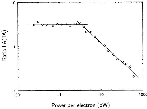
FIG. 3. Ratio of LA- to TA-mode peak heights vs power. The straight lines are shown as a guide to the eye.
