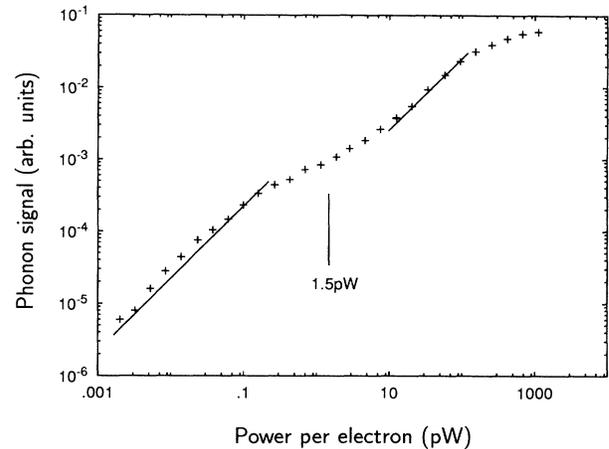
FIG. 2. TA-mode signal height vs input power. The break at 1.5 pW per electron has been shown previously in the heterojunction system to occur for a carrier temperatures around 50 K and is associated with the onset of LO mode emission. The flattening off above approximately 100 pW per electron is due to bolometer saturation.
