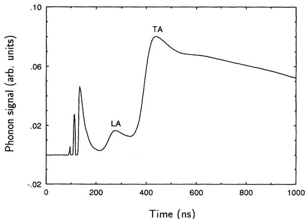
FIG. 1. Typical phonon time-of-flight trace taken in the optical emission regime (100 pW per electron) showing the characteristic TA peak tail of phonons arriving later than the ballistic flight time.
