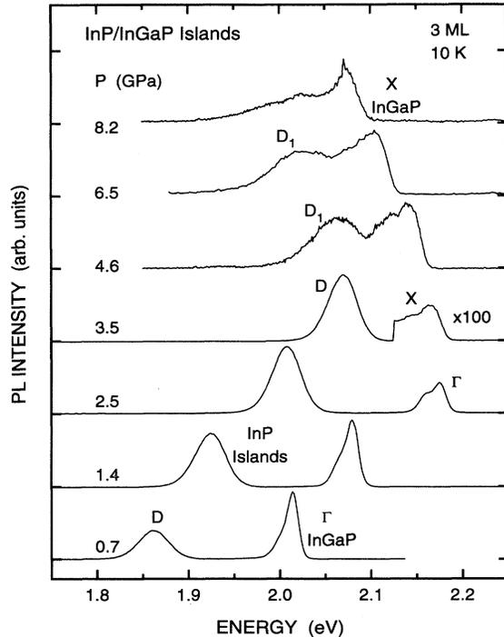
FIG. 2. PL spectra of the 3 ML InP island sample for different pressures. Each spectrum has been normalized to the maximum intensity, except for the part of the 3.5 GPa spectrum.
