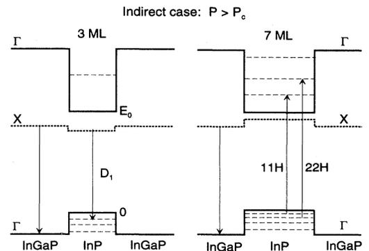
FIG. 4. Sketch of the  $\Gamma$ - and  $X$ -point conduction-band and  $\Gamma$ -point valence-band profile of the  $\text{InP}$  islands above the  $\Gamma$ - $X$  crossover pressure. Arrows indicate the assignment of the observed optical transitions.
