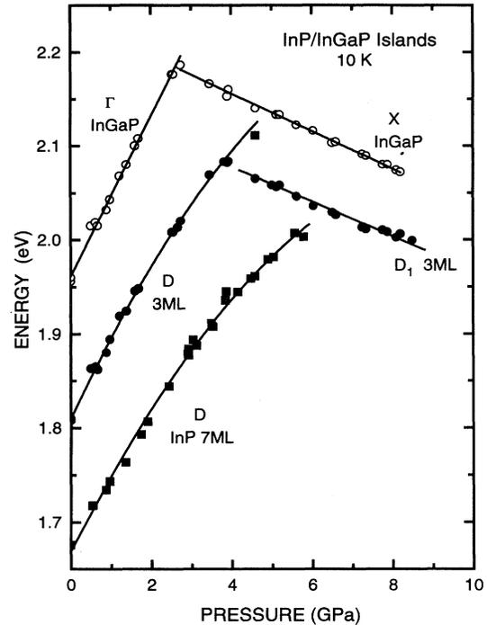
FIG. 3. Pressure dependence of the energy of PL peaks for the 3 ML and 7 ML InP island samples.
