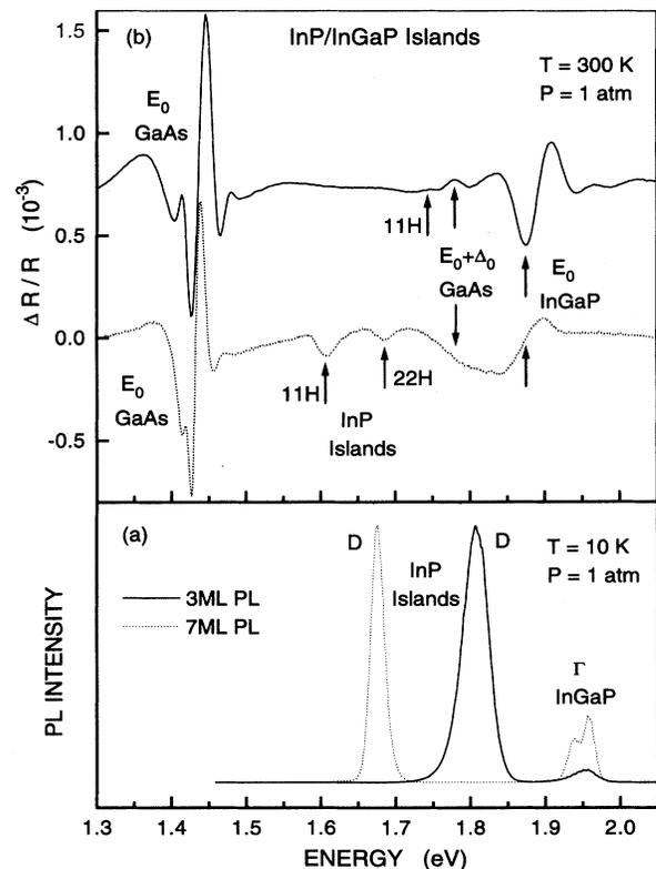
FIG. 1. (a) Ambient pressure photoluminescence spectra at 10 K and (b) photoreflectance spectra at 300 K of  $\text{InP}/\text{In}_x\text{Ga}_{1-x}\text{P}$  island samples grown with 3 ML (solid lines) and 7 ML (dotted lines) nominal thickness.
