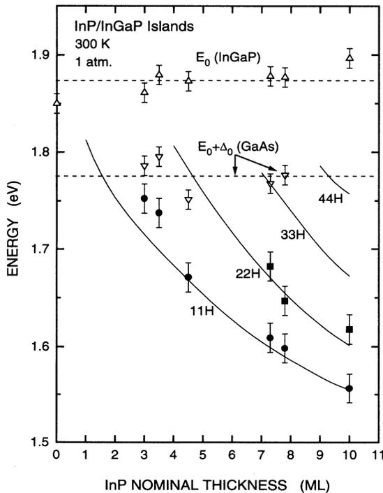
FIG. 5. Measured (symbols) and calculated (solid lines) energies for the optical transitions observed in PR spectra of samples with different nominal InP growth thickness of the islands.
