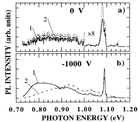
FIG. 5. Photoluminescence spectra of the undoped reference Si epilayers grown with different bias applied to the substrate: (a) zero bias and (b) negative bias at  $-1000$  V. Spectra of the as-grown and the hydrogen-treated samples are shown by the solid and the dashed curves, respectively. The dip around 0.90 eV appearing in all spectra corresponds to the absorption by the water vapor.
