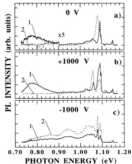
FIG. 1. Photoluminescence spectra of the B-doped Si epilayers grown with different bias applied to the substrate: (a) zero bias, (b) positive bias at +1000 V, and (c) negative bias at –1000 V. Spectra of the as-grown and the hydrogen-treated samples are shown by the solid and the dashed curves, respectively. The dip around 0.90 eV appearing in all spectra corresponds to the absorption by the water vapor.
