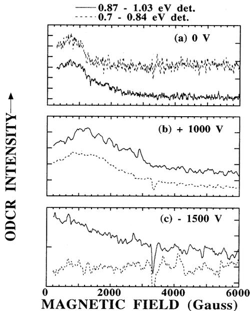
FIG. 4. ODCR spectra monitored in two different spectral ranges from the B-doped samples grown with (a) zero bias, (b) positive bias, and (c) negative bias. The solid and dashed curves were obtained by monitoring the PL emissions in the spectral range 0.87–1.03 and 0.70–0.84 eV, respectively.
