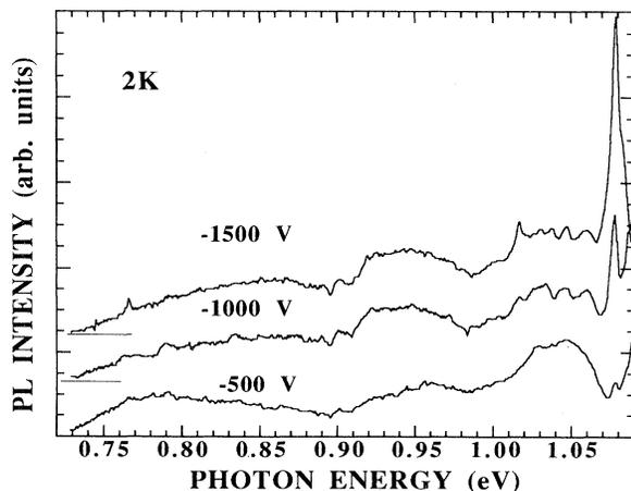
FIG. 2. PL spectra of the B-doped Si epilayers as a function of an increasing negative bias applied to the substrate during the MBE growth. The dip around 0.90 eV appearing in all spectra corresponds to the absorption by the water vapor.
