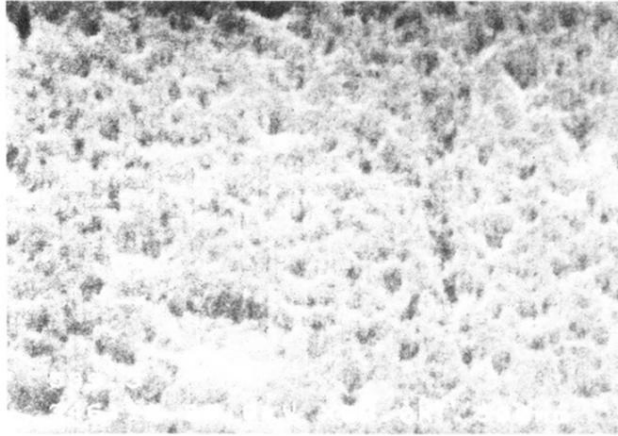
FIG. 3. SEM image of the top view of a p -type \text{Si}_{0.95}\text{Ge}_{0.05} layer. The width of the shown sample area corresponds to 2\ \mu\text{m} .
