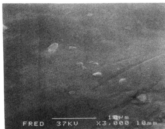
FIG. 3. SEM pictures of the surface of sample 3 after polishing (see text for details): (top) 100- \mu\text{m} scale and (bottom) 10- \mu\text{m} scale. Evidently, the surface defects seen in Fig. 2 do not penetrate into the bulk of the sample.
