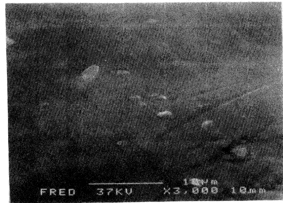
FIG. 3. SEM pictures of the surface of sample 3 after polishing (see text for details): (top) 100- \mu\text{m} scale and (bottom) 10- \mu\text{m} scale. Evidently, the surface defects seen in Fig. 2 do not penetrate into the bulk of the sample.
