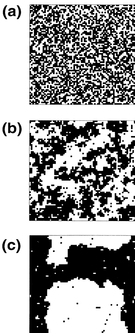
FIG. 14. Calculated As unit distribution on surfaces with a coverage of 0.5 in the transition from As-covered to In-exposed surfaces with (a) E_s=2.5 eV, E_i=0.0 eV, (b) E_s=2.3 eV, E_i=0.1 eV, and (c) E_s=2.18 eV, E_i=0.16 eV. The black domains correspond to As-covered sites and the white domains correspond to In-exposed sites.
