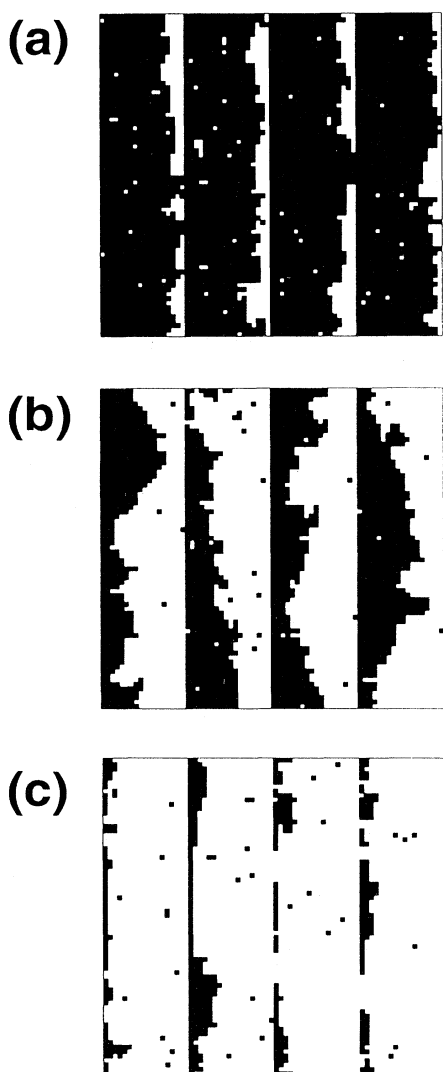
FIG. 22. Calculated As-unit distribution on a misoriented surface with a terrace size of 18 As units during the transition at temperatures of (a) 446 °C, (b) 448 °C, and (c) 449 °C for E_s=2.18 eV and E_i=0.16 eV. The black domains correspond to As-covered sites and the white domains correspond to In-exposed sites.
