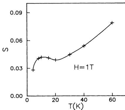
FIG. 4. Normalized flux-creep rate  $S$  vs  $T$ . The solid line (cubic spline fitting) is a guide to the eye.
