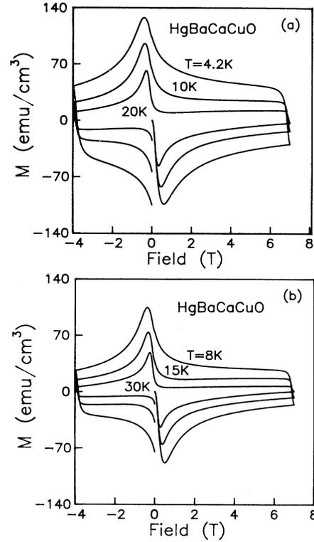
FIG. 1. Magnetization loops of the Hg-1223 sample at 4.2, 8, 10, 15, 20, and 40 K.
