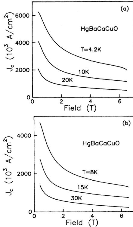
FIG. 5. Field dependence of critical current densities for the Hg-1223 sample.
