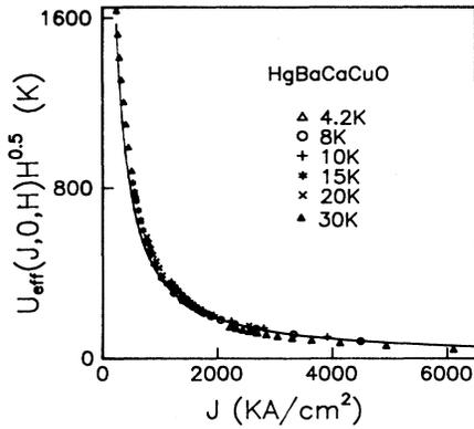
FIG. 8. Current density dependence of effective activation energy  $U_{\text{eff}}(J, 0, H=1 \text{ T})$  deduced from the magnetic hysteresis loops.  $U_{\text{eff}}(J, T, H) = kG(T)U_{\text{eff}}(J, 0, H=1 \text{ T})/H^n$ , with the fitting parameter  $n=0.5$ . The solid line is the power-law fitting curve in Fig 7(a).
