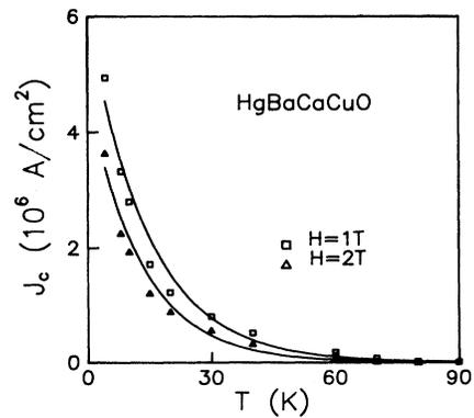
FIG. 6.  $J_c(T)$  of the Hg-1223 sample at 1 and 2 T, estimated from the Bean model, displays a drastic drop with temperature. The solid line is an exponential fit with form  $e^{-T/T_0}$ , where  $T_0 \approx 15$  and 13 K for  $H=1$  and 2 T, respectively.
