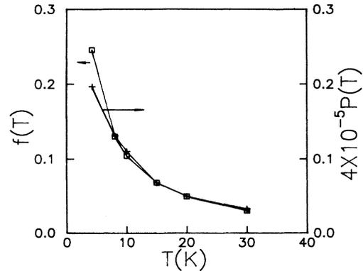
FIG. 10. Scale of  $P(T)$  with  $f(T) = [T/G(T)]^{-1/\mu}$ , where  $G(T) = \{1 - [T/T_{\text{irr}}(H)]^2\}^{3/2}$ ,  $T_{\text{irr}}(H=1 \text{ T}) = 87 \text{ K}$  and  $\mu = 1.03$ .  $P(T)$  is the coefficient in  $J(H) = P(T)H^{-Q}$ , in which  $J(H)$  and  $H$  are in the units of  $\text{kA/cm}^2$  and T, respectively.
