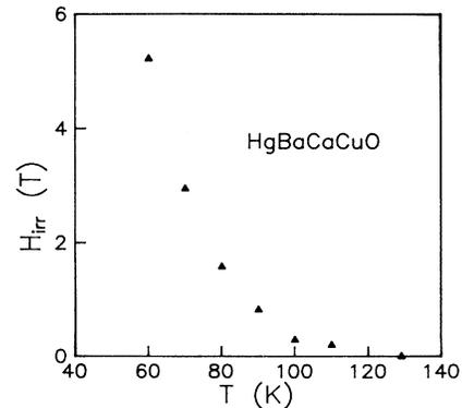
FIG. 2. Irreversibility field ( $H_{\text{irr}}$ ) plotted against temperature  $T$  for the Hg-1223 sample. The criterion of  $J_c$  is  $10^4 \text{ A/cm}^2$ . In the field range from 0.5 to 5.2 T,  $T$  depends on  $H_{\text{irr}}$  logarithmically,  $T = 87.1 - 16.1 \ln H_{\text{irr}}$ .
