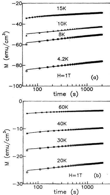
FIG. 3. Magnetization relaxations of the Hg-1223 sample at temperatures of 4.2, 8, 10, 15, 20, 30, 40, and 60 K and field of 1 T display a logarithmic decay (solid lines).
