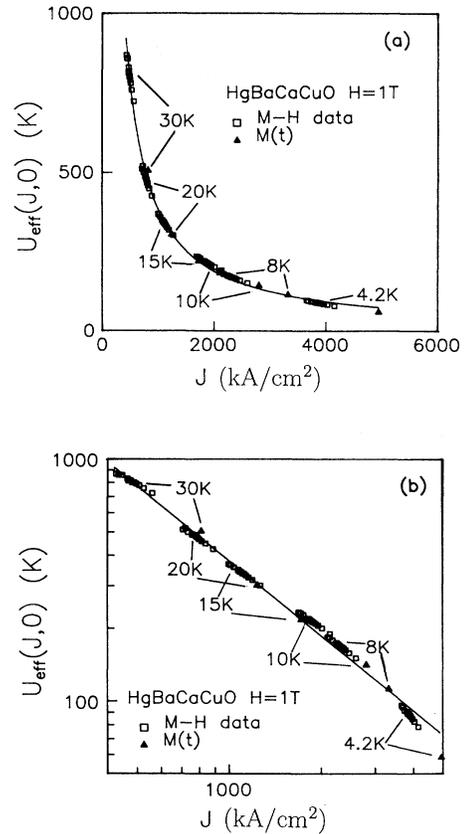
FIG. 7(a) The effective activation energies  $U_{\text{eff}}(J, 0, H=1 \text{ T})$  ( $\square$ ) extracted from the magnetic relaxation fits a power law (solid line is the result of best fitting). The data points marked with ( $\blacktriangle$ ) are those based on the width of magnetic hysteresis loops at  $H=1 \text{ T}$ . The fitting parameter  $C=16$ . (b) A double-logarithmic plot of  $U_{\text{eff}}(J, 0, H=1 \text{ T})$  indicating a power-law dependence on the current density.
