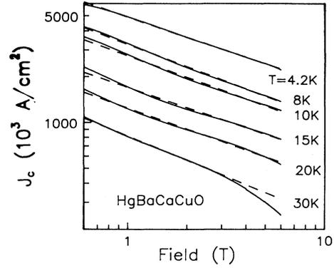
FIG. 9. Double-logarithmic plot magnetic critical current  $J_c$  as a function of field at several temperatures. The dashed lines are best fits with power law  $J(H) = P(T)H^{-Q}$ , where  $Q = 0.44, 0.49, 0.47, 0.44, 0.46$ , and  $0.53$  for data of  $T = 4.2, 8, 10, 15, 20$ , and  $30 \text{ K}$ , respectively; namely, the slopes of the lines in the figure are approximately equal.
