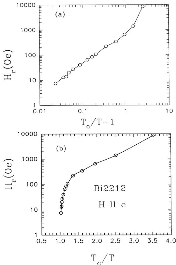
FIG. 7. Plot of  $H_r$  values vs (a)  $(T_c/T - 1)$  and (b)  $T_c/T$ , respectively.
