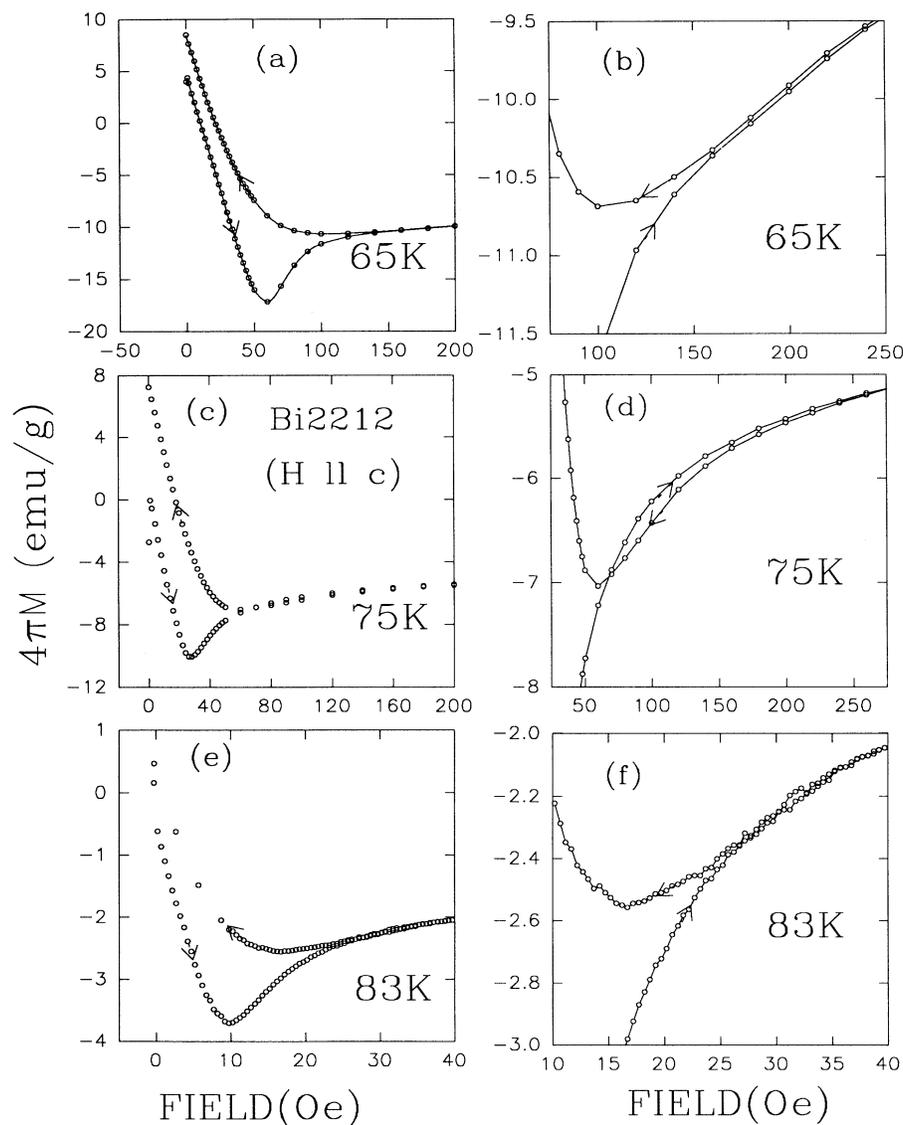
FIG. 4. Magnetization hysteresis curves in Bi2212 for  $\mathbf{H}\parallel c$  at 65 K, 75 K, and 83 K, respectively. For each temperature, the behavior near the corresponding  $H_r(T)$  value has been shown on an expanded scale. An anomalous behavior may be noted at 75 K in (d) where the ZFC magnetization curve lies above the reversed magnetization curve for  $H > 75$  Oe.
