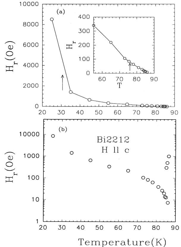
FIG. 6. The variation of irreversibility field ( $H_r$ ) values with temperature on (a) linear and (b) log scales, respectively. The arrows in (a) mark the temperatures around which signatures of the two-component magnetic response are visible.
