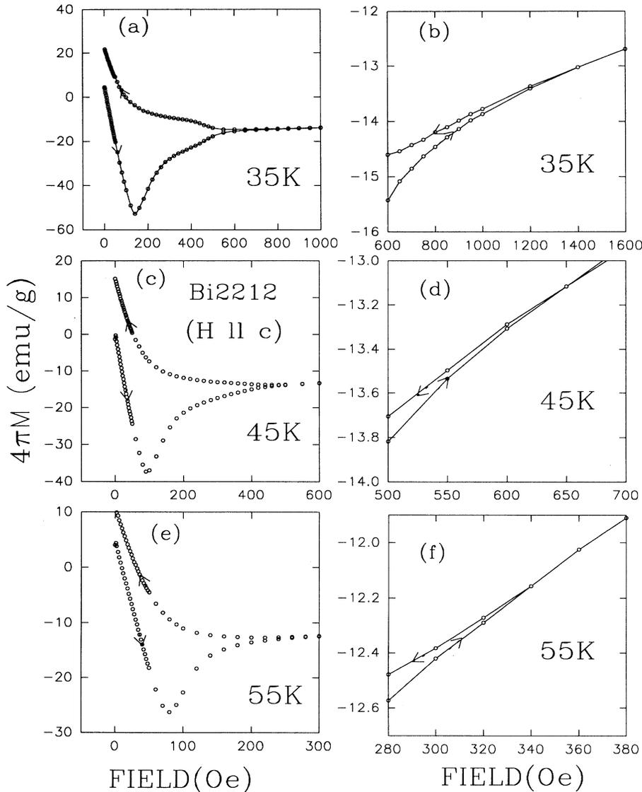
FIG. 3. Magnetization hysteresis curves in Bi2212 for  $\mathbf{H} \parallel c$  at 35 K, 45 K, and 55 K, respectively. For each temperature, the behavior near the corresponding  $H_r(T)$  value has also been shown on an expanded scale.
