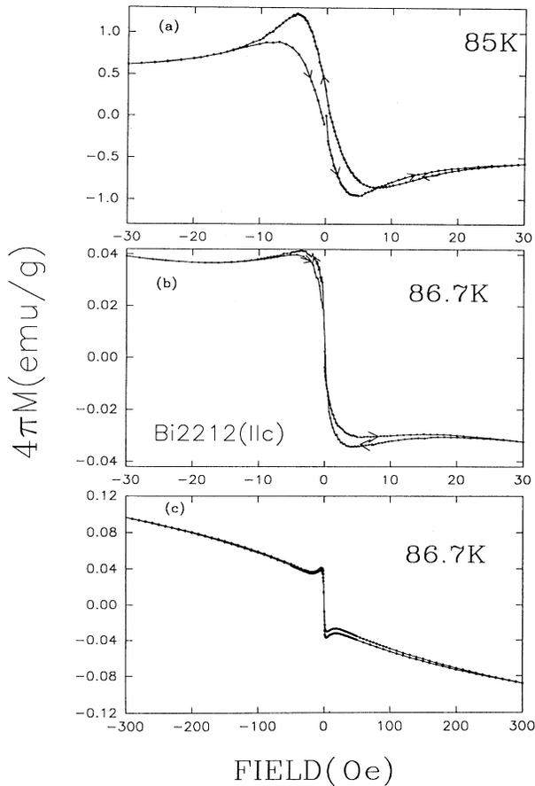
FIG. 5. Magnetization hysteresis loops in Bi2212 for  $\mathbf{H} \parallel c$  at 85 K and 86.7 K. The ZFC magnetization leg lies above the reversed magnetization leg over the entire field region ( $0 < H < 30$  Oe) at 86.7 K (b), whereas at 85 K, the anomalous behavior is evident only for  $H > 8$  Oe. The magnetization loop between  $\pm 300$  Oe at 86.7 K (c) has an unusual shape, corresponding to a two-component magnetic response as described in Ref. 7.
