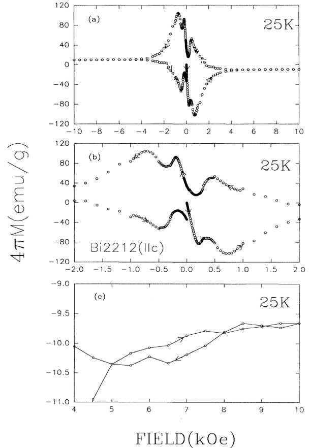
FIG. 2. Magnetization hysteresis curves in Bi2212 for  $H \parallel c$  at 25 K. (b) and (c) show the details on the expanded scales across the  $H=0$  region and on reversal from  $H_{\max}$  of 10 kOe, respectively.
