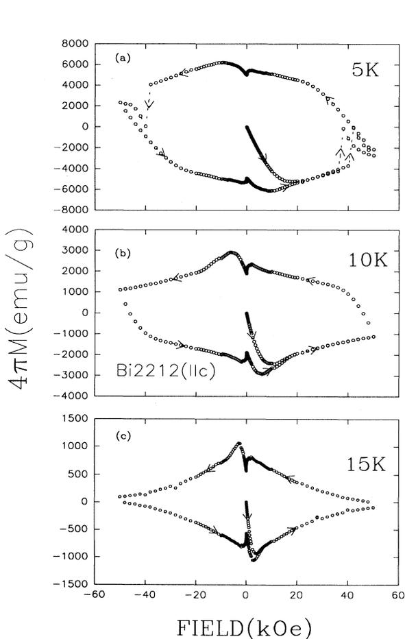
FIG. 1. Magnetization hysteresis loops for  $H \parallel c$  in Bi2212 at 5 K, 10 K, and 15 K, respectively.
