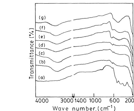
FIG. 5. Room-temperature infrared spectra of several samples: (a) crystalline Bi<sub>2</sub>O<sub>3</sub>, (b) 27.15 mol % CuO, (c) 35.35 mol % CuO, (d) 45.70 mol % CuO, (e) 55.62 mol % CuO, (f) 67.60 mol % CuO, and (g) crystalline CuO.
