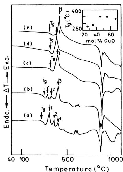
FIG. 4. Differential thermal analysis curves of several samples: (a) 27.15 mol % CuO, (b) 35.35 mol % CuO, (c) 45.70 mol % CuO, (d) 55.62 mol % CuO, and (e) 67.60 mol % CuO. ↓ indicated by T<sub>g</sub> is the glass transition temperature and ↓1, ↓2, etc. indicate crystallization temperatures. Inset shows glass transition temperature (T<sub>g</sub>) as a function of CuO content.
