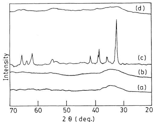
FIG. 1. X-ray diffractograms of several samples: (a) 27.15 mol % CuO, (b) 45.70 mol % CuO, (c) 45.70 mol % CuO heat treated at 500°C for 20 h, and (d) 67.60 mol % CuO.
