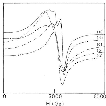
FIG. 6. Room-temperature ESR spectra of bismuth cuprate glasses recorded at a microwave frequency 9.44 GHz. (a) 27.15 mol % CuO (gain =  $2.5 \times 10^3$ ), (b) 35.35 mol % CuO (gain =  $4.0 \times 10^3$ ), (c) 45.70 mol % CuO (gain =  $8.0 \times 10^3$ ), (d) 55.62 mol % CuO (gain =  $5.0 \times 10^3$ ), and (e) 67.60 mol % CuO (gain =  $6.3 \times 10^3$ ).
