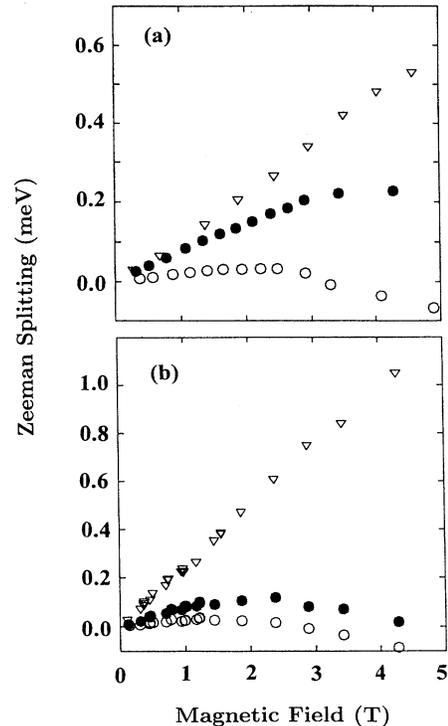
FIG. 2. (a) Zeeman splitting for  $x=0.075$  for well widths of 12 ( $\nabla$ ), 8 ( $\bullet$ ), and 4 nm ( $\circ$ ). (b) Zeeman splittings for  $x=0.11$  for well widths of 10 ( $\nabla$ ), 6 ( $\bullet$ ), and 3 nm ( $\circ$ ).
