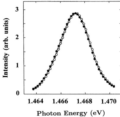
FIG. 1. Zeeman components of the heavy-hole exciton luminescence observed in  $\sigma^+$  ( $\circ$ ) and  $\sigma^-$  ( $\bullet$ ) polarization for well width 8 nm, indium concentration 0.075, applied field  $B_z=1.07$  T, and temperature 1.7 K.
