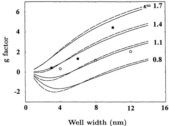
FIG. 3. Experimental (points) and calculated (curves) exciton  $g$  factors; closed circles and solid curves for  $x=0.75$ , open circles and dashed curves for  $x=0.11$ . Calculations are shown for a range of values of Luttinger  $\kappa$  in the  $\text{In}_x\text{Ga}_{1-x}\text{As}$  well and comparison with the experimental points leads to the values quoted in the text and plotted in Fig. 4.
