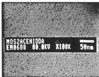
FIG. 1. TEM micrograph showing 3-nm MoS 2 clusters.
