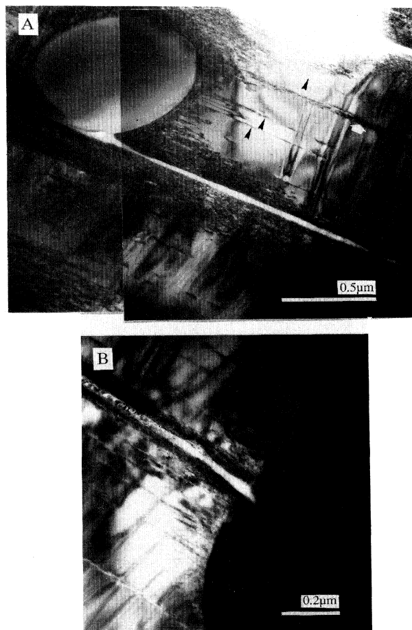
FIG. 4. Interaction of a microcrack with a 211 precipitate with associated thick degraded layers viewed along the [100] direction: (a) aged sample, oxygenated for 156 h, and (b) nonaged sample, oxygenated for 60 h.
