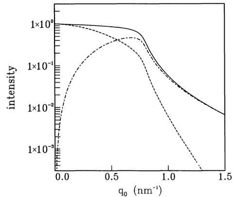
FIG. 2. Coherent and incoherent reflectivity vs wave-vector transfer, calculated with the Rayleigh method for Cu  $K\alpha_1$  radiation on gold with rms roughness  $\sigma = 1.5 \text{ nm}$  and large correlation length  $\xi$ . Long dashes: coherent reflectivity  $|r_k|^2$  [Eq. (12)]; dash-dotted line: integrated incoherent reflection [Eq. (15)]; solid line: sum of coherent and incoherent reflection (or  $|r_k|^2, \sigma = 0$ ).
