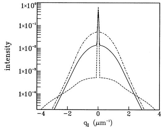
FIG. 5. Coherent and incoherent reflectivity vs parallel wave-vector transfer in a transverse scan at  $q_0=0.6$  nm<sup>-1</sup>, calculated for Cu  $K\alpha_1$  radiation on gold with rms roughness  $\sigma=1.5$  nm and two different correlation lengths  $\xi$ . Dashed line:  $\xi=20$  nm (DWBA); dash-dotted line:  $\xi=2$   $\mu$ m (DWBA); solid line:  $\xi=2$   $\mu$ m (Rayleigh method).
