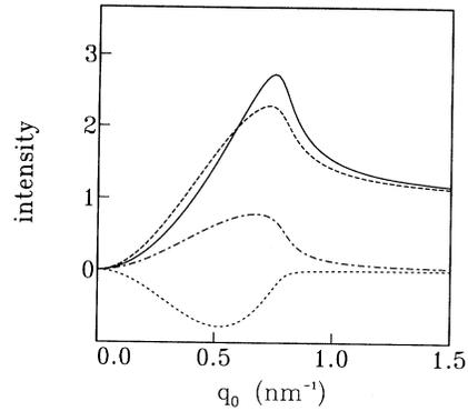
FIG. 4. Coherent and incoherent transmission factor  $Tk_0/k_1'$  vs wave-vector transfer, calculated with the Rayleigh method for Cu  $K\alpha_1$  radiation in gold with rms roughness  $\sigma=1.5$  nm and large correlation length  $\xi$ . Long dashes: coherent transmission  $|\tilde{t}_k|^2$  [Eq. (13)]; dash-dotted line: incoherent transmission [Eq. (7)]; short dashes: correction for absorption in rough interfacial layer; solid line: total transmission (or  $|t_k|^2, \sigma=0$ ).
