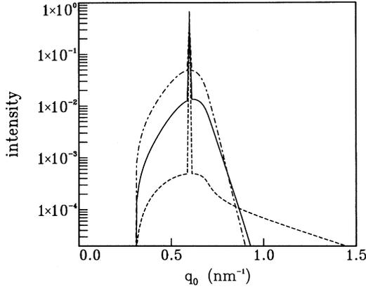
FIG. 6. Coherent and incoherent reflectivity vs perpendicular wave-vector transfer in a detector scan at  $k_0=0.3 \text{ nm}^{-1}$ , calculated for Cu  $K\alpha_1$  radiation on gold with rms roughness  $\sigma=1.5 \text{ nm}$  and two different correlation lengths  $\xi$ . Dashed line:  $\xi=20 \text{ nm}$  (DWBA); dash-dotted line:  $\xi=2 \mu\text{m}$  (DWBA); solid line:  $\xi=2 \mu\text{m}$  (Rayleigh method).
