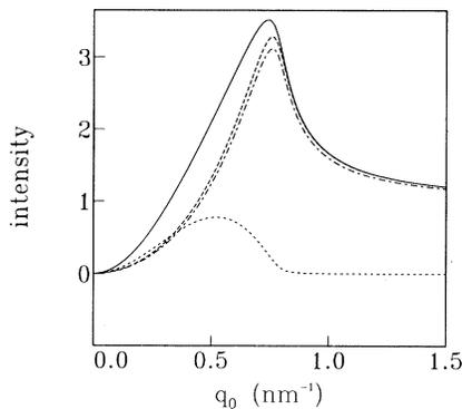
FIG. 3. Coherent and incoherent transmission factor  $Tk_0/k_1'$  vs wave-vector transfer, calculated in the DWBA for Cu  $K\alpha_1$  radiation on gold with rms roughness  $\sigma=1.5$  nm and small correlation length  $\xi$ . Long dashes: coherent transmission  $|\tilde{t}_k|^2$  [Eq. (2)]; dash-dotted line: coherent transmission according to Caticha (Ref. 11) (see text); short dashes: absorption in rough interfacial layer; solid line: total transmission.
