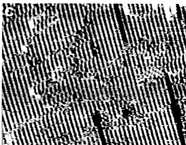
FIG. 12. Lifting of the c(2 \times 2) structure for small tunneling resistances on Au(110) with \theta_K \approx 0.35 ML, adsorbed at T \approx 490 K. (a) R_t = 2000 MΩ ( U = -789 mV, I = 0.4 nA); (b) R_t = 30 MΩ ( U = -489 mV, I = 16 nA); (c) R_t = 12 MΩ ( U = -489 mV, I = 40 nA) (each 350 \times 200 Å 2 ).
