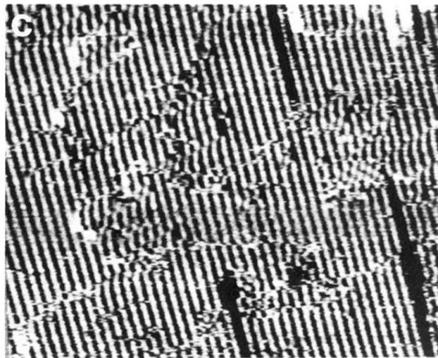
FIG. 12. Lifting of the c(2 \times 2) structure for small tunneling resistances on Au(110) with \theta_K \approx 0.35 ML, adsorbed at T \approx 490 K. (a) R_t = 2000 \text{ M}\Omega ( U = -789 \text{ mV} , I = 0.4 \text{ nA} ); (b) R_t = 30 \text{ M}\Omega ( U = -489 \text{ mV} , I = 16 \text{ nA} ); (c) R_t = 12 \text{ M}\Omega ( U = -489 \text{ mV} , I = 40 \text{ nA} ) (each 350 \times 200 \text{ \AA}^2 ).
