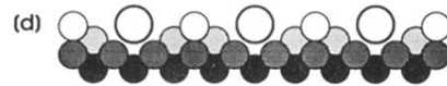
FIG. 2. (a) STM image of the Au(110) surface for \theta_K \approx 0.08 ML (annealed to 950 K): K-induced (1 \times 3) reconstruction with single (1 \times 2) troughs ( 610 \times 510 \text{ \AA}^2 ); (b) STM contour along the marked line in (a); (c) model of the K-induced (1 \times 3) phase on Au(110), top view; (d) side view.
