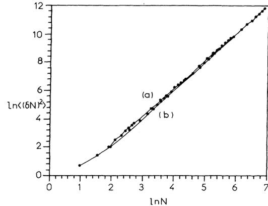
FIG. 3. The novel relation  $\langle[\delta N(E)]^2\rangle \propto \langle N(E)\rangle^2$  is shown to be valid both (a) for the percolation cluster and (b) for the percolation backbone. The small difference in the slopes lies in the slightly reduced value of  $d_s$  for the percolation backbone.
