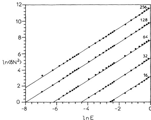
FIG. 2. The same as Fig. 1 but for the number variance  $\langle[\delta N(E)]^2\rangle$  as a function of the energy  $E$ . The solid lines are the best fits to the data and their slopes are found to be equal to  $d_s$ , establishing the law:  $\langle[\delta N(E)]^2\rangle \propto \langle N(E)\rangle^2$ .
