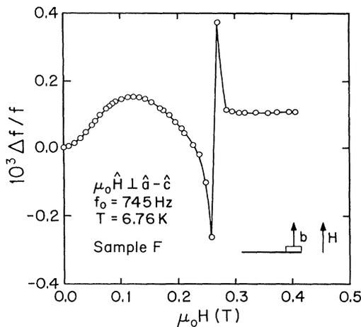
FIG. 4. Relative frequency shift  $\Delta f/f$  and inverse quality factor  $1/Q$  versus magnetic field  $\mu_0 H$  for sample F in the transverse orientation (see inset) at  $T=6.76$  K. The line is a guide to illustrate a discontinuity.
