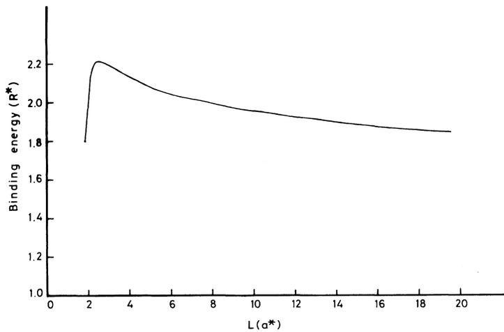
FIG. 1. Variation of the binding energy of a hydrogenic donor at the center of the  $|z|^{2/3}$  quantum well as a function of well width  $L$ , having a barrier height  $V_0 = 220.23$  meV.
