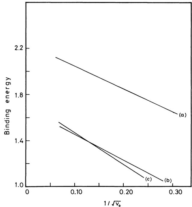
FIG. 2. Variation of the binding energy (in effective Rydbergs) as a function of  $1/\sqrt{V_0}$  where  $V_0$  is expressed in effective Rydbergs in the  $|z|^{2/3}$  quantum well of width  $L = 1024 \text{ \AA}$ : curve  $a$  for a hydrogenic donor at the center of the well, curve  $b$  for a heavy-hole exciton, and curve  $c$  for a light-hole exciton.
