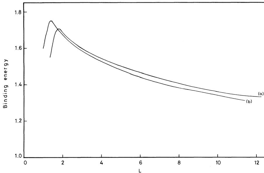
FIG. 3. Variation of the binding energy (in effective Rydbergs) as a function of well width  $L$  (in units of the effective Bohr radius) in the  $|z|^{2/3}$  quantum well having a barrier height  $V_0=220.23$  meV for electrons and  $V_0=118.59$  meV for holes: curve  $a$  for a heavy-hole exciton and curve  $b$  for a light-hole exciton.
