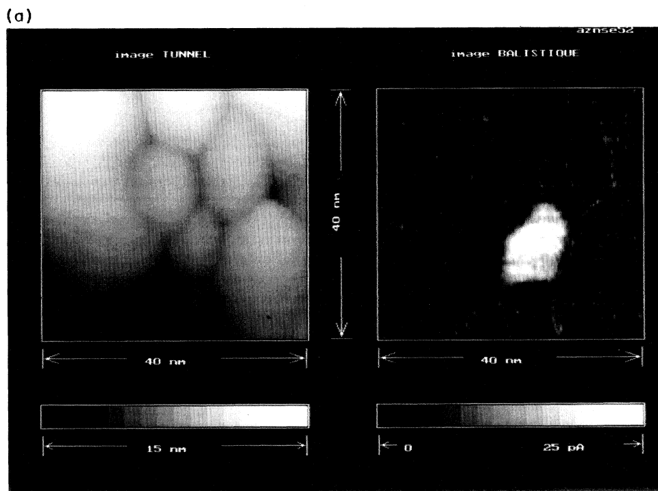
FIG. 5. (a) STM topography (left) and BEEM image (right) of the Schottky junction. The scanned surface is 40 \times 40 nm 2 ( I_{\text{tunnel}} = 25 nA, V_s = 2.5 V). The maximum contrast of the BEEM image corresponds to collector current variations of 25 pA. (b) Experimental BEEM spectrum realized on the bright area of (a). The calculations yield a Schottky-barrier height of 2.10 eV (solid line).
