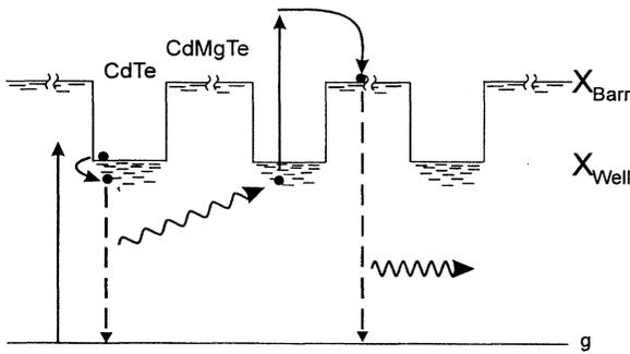
FIG. 3. Schematic illustration of the excitation scenario underlying the observed anti-Stokes photoluminescence. The horizontal solid lines represent the lowest exciton states in the barrier ( $X_{\text{Barr}}$ ), the lowest, confined exciton states in the quantum well ( $X_{\text{Well}}$ ), and the crystal ground state ( $g$ ). Short horizontal lines indicate the presence of localized exciton states.
