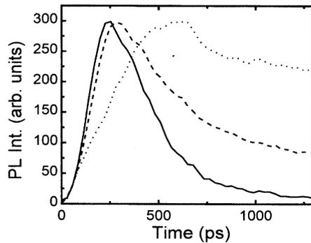
FIG. 4. Time-resolved PL spectra of the MQW sample with  $L_B = 144$  nm; solid curve: QW PL; dashed curve: barrier PL excited by a frequency doubled Ti:sapphire laser at  $\approx 400$  nm; dotted curve: anti-Stokes barrier PL excited at the lowest hh exciton resonance of the QW. All spectra are normalized.
