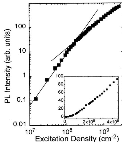
FIG. 2. Double-logarithmic plot of the density dependence of the anti-Stokes PL at 10 K. Linear regressions yield slopes of 2.1 and 1.08 for densities below and above  $2 \times 10^8$   $\text{cm}^{-2}$ , respectively. The inset shows a linear plot for low excitation densities.
