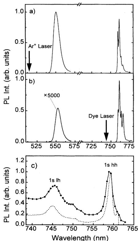
FIG. 1. (a),(b) Time-integrated PL spectra of the MQW with a barrier thickness of  $L_B = 144$  nm at 10 K (a) excited above the barrier and (b) below the barrier. (c) Corresponding QW PLE spectrum (dashed curve) and anti-Stokes barrier PLE spectrum (solid curve) (both normalized to the respective maximum intensity at the 1s heavy-hole exciton resonance).
