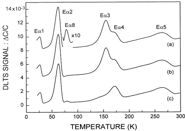
FIG. 1. DLTS spectra of  $\alpha$ -particle-irradiated  $n$ -type GaAs ( $f=1$  Hz,  $V_r=2$  V, and  $V_p=1.9$  V): (a) after reverse-bias (2-V) cooling; (b) after zero-bias cooling; (c) after applying a forward current density of  $5.6$  A  $\text{cm}^{-2}$  at  $105$  K for  $10$  s.
