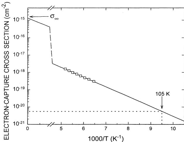
FIG. 2. Variation of  $E\alpha 3$  electron-capture cross-section as function of temperature. Measurement conditions:  $V_r=4$  V and  $V_p=4.2$  V.
