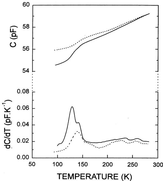
FIG. 4. TSCAP ( $C$  vs  $T$ ) and  $dC/dT$  vs  $T$  of OMVPE-grown  $1.2 \times 10^{16} \text{ cm}^{-3}$  doped *n*-type GaAs, irradiated with  $\alpha$  particles. The capacitance was recorded at a scan rate of  $3 \text{ K min}^{-1}$ . —, zero-bias cooldown, then scan up with  $V_f = 4 \text{ V}$ . - - -, zero-bias cooldown followed by the application of an injection pulse, then scan up with  $V_f = 4 \text{ V}$ .
