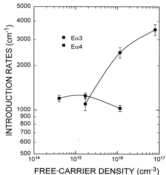
FIG. 6. Change in  $E\alpha 3$  and  $E\alpha 4$  introduction rates as a function of free-carrier concentration for Si-doped  $n$ -type GaAs.
