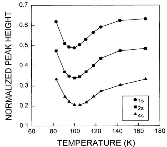
FIG. 3. Change in  $E\alpha 3$  peak height as a function of temperature when a forward current is applied at a current density of  $1.4$  A  $\text{cm}^{-2}$  for times  $1$ ,  $2$ , and  $4$  s.
