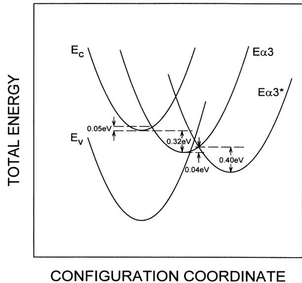
FIG. 5. Configuration-coordinate ( $C$ - $C$ ) diagram for the  $E\alpha 3$  defect.
