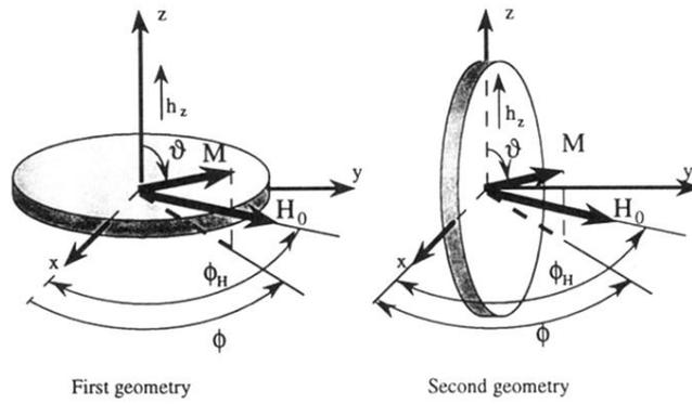
FIG. 1. Two different possible orientations of the magnetization ( $\mathbf{M}$ ), the static magnetic field ( $\mathbf{H}_0$ ), and the hyperfrequency magnetic field ( $\mathbf{h}_z$ ) in strain-modulated ferromagnetic resonance experiments.
