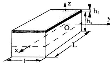
FIG. 2. Definition of the axes in an experiment for observing the deflection of a magnetostrictive bimorph.
