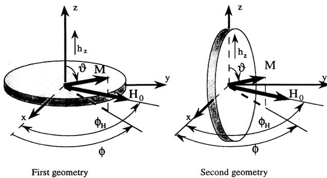
FIG. 1. Two different possible orientations of the magnetization ( $\mathbf{M}$ ), the static magnetic field ( $\mathbf{H}_0$ ), and the hyperfrequency magnetic field ( $\mathbf{h}_z$ ) in strain-modulated ferromagnetic resonance experiments.
