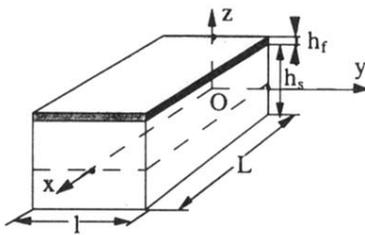
FIG. 2. Definition of the axes in an experiment for observing the deflection of a magnetostrictive bimorph.
