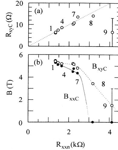
FIG. 5. (a)  $R_{xyC}$  is plotted against  $R_{xxn}$ . (b) Dependence of the critical fields  $B_{xxC}$  (solid circles) and  $B_{xyC}$  (open circles) on  $R_{xxn}$  for the nine films studied. The region  $B_{xxC} < B < B_{xyC}$  corresponds to the unusual insulating phase.
