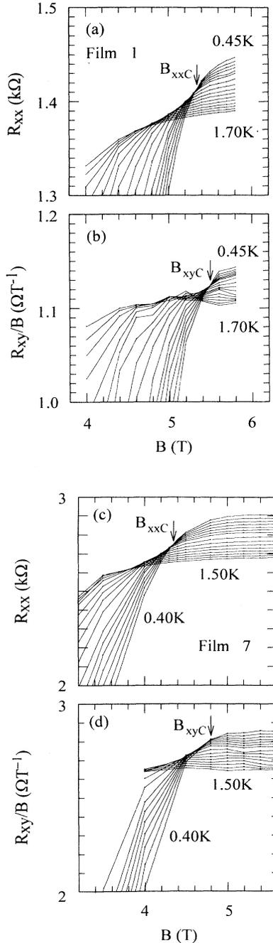
FIG. 2. Magnetic-field dependence of (a)  $R_{xx}$  and (b)  $R_{xy}/B$  for film 1, and that of (c)  $R_{xx}$  and (d)  $R_{xy}/B$  for film 7, at various temperatures. Isotherms range from 0.45 to 1.70 K for film 1 and from 0.40 to 1.50 K for film 7 in 0.05 K steps below 0.70 K and in 0.10 K steps above 0.70 K.
