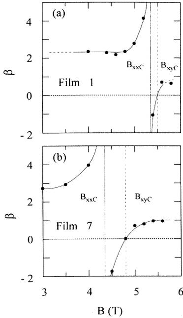
FIG. 4. Magnetic-field dependence of the exponent  $\beta(B)$  in Eq. (1) for (a) film 1 and (b) film 7. Vertical solid and broken lines represent  $B_{xxC}$  and  $B_{xyC}$ , respectively. The region where  $\beta(B)$  is negative ( $B_{xxC} < B < B_{xyC}$ ) corresponds to the distinct insulating phase.
