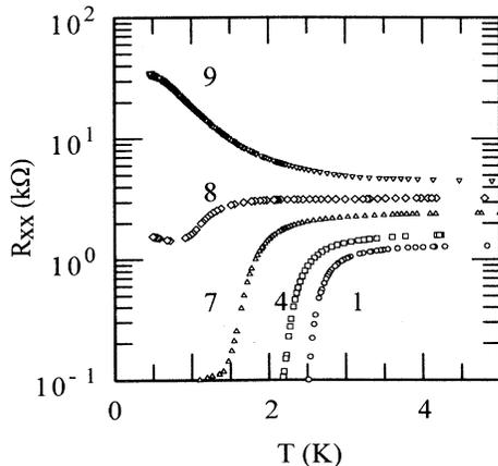
FIG. 1. Temperature dependence of the sheet resistance  $R_{xx}(T)$  for five selected films.
