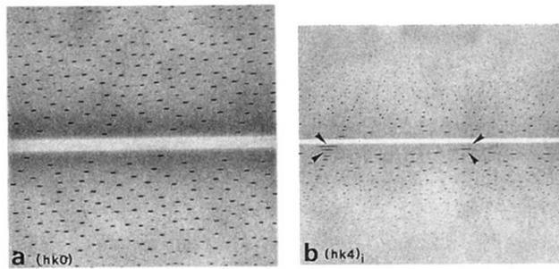
FIG. 3. X-ray diffraction Weissenberg photographs at 295 K of  $\text{Cu}_{0.25}\text{Ni}_{0.75}(\text{pc})\text{I}$ : (a) zeroth-level Weissenberg photograph ( $hk0$ ) common to the organic and iodine sublattices and (b) fourth-level Weissenberg photograph of iodine sublattice ( $hk4$ )<sub>I</sub>. In (b) the arrows point towards the equivalent Bragg reflections belonging to the reciprocal space of the four domains discussed in the text.
