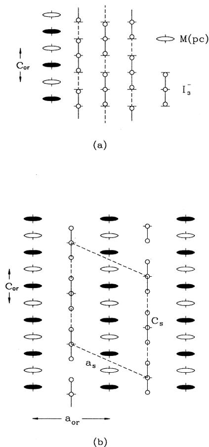
FIG. 1. (a) Disorder model for the iodine chains in  $M(\text{pc})\text{I}$  according to Ref. 12. The three possible iodine chain arrangements are shown on the right. The  $M(\text{pc})$  stack is shown on the left. White and black ellipses refer to the two  $M(\text{pc})$  molecules staggered by  $40^\circ$ . (b) Projection of the ordered lattice along  $b_s = b_{\text{or}}$ ;  $a_s = a_{\text{or}} + c_{\text{or}}$ ;  $c_s = 3c_{\text{or}}$ .
