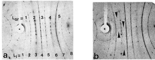
FIG. 2. Fixed-film fixed-crystal x-ray diffraction pattern for the crystal  $\text{Cu}_{0.75}\text{Ni}_{0.25}(\text{pc})\text{I}$  at (a) 295 K and (b) 20 K. In (a) the layers of Bragg reflections perpendicular to the  $c$  direction are labeled according to the organic ( $l_{or}$ ) and iodine ( $l_I$ ) sublattice reciprocal periods. In (b) the arrows point towards Bragg reflections due to the intermodulation of the  $M(\text{pc})$  and  $\text{I}_3^-$  sublattices.
