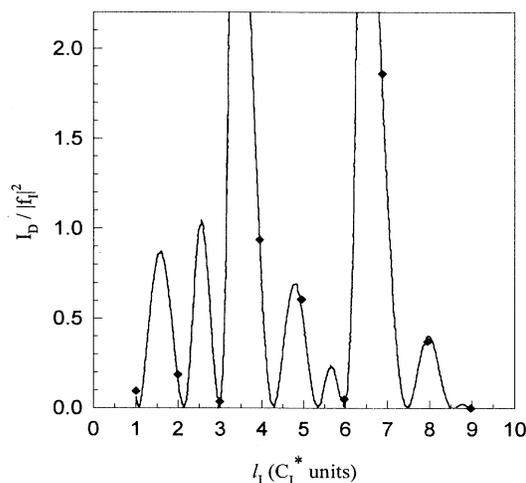
FIG. 5. Dependence of the reduced iodine diffuse intensity  $I_D/|f_1|^2$  as a function of the iodine Miller index  $l_1$ . The data are shown by a dot at each integer  $l_1$  value and the continuous line is the fit given by expression (1).
