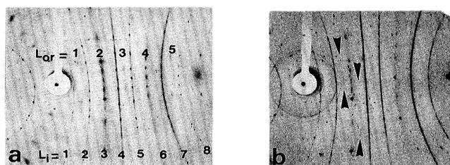
FIG. 2. Fixed-film fixed-crystal x-ray diffraction pattern for the crystal  $\text{Cu}_{0.75}\text{Ni}_{0.25}(\text{pc})\text{I}$  at (a) 295 K and (b) 20 K. In (a) the layers of Bragg reflections perpendicular to the  $c$  direction are labeled according to the organic ( $l_{\text{or}}$ ) and iodine ( $l_{\text{I}}$ ) sublattice reciprocal periods. In (b) the arrows point towards Bragg reflections due to the intermodulation of the  $M(\text{pc})$  and  $\text{I}_3^-$  sublattices.
